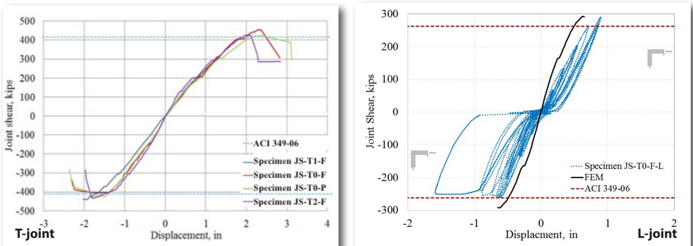
Figure 3: Joint shear – displacement responses
