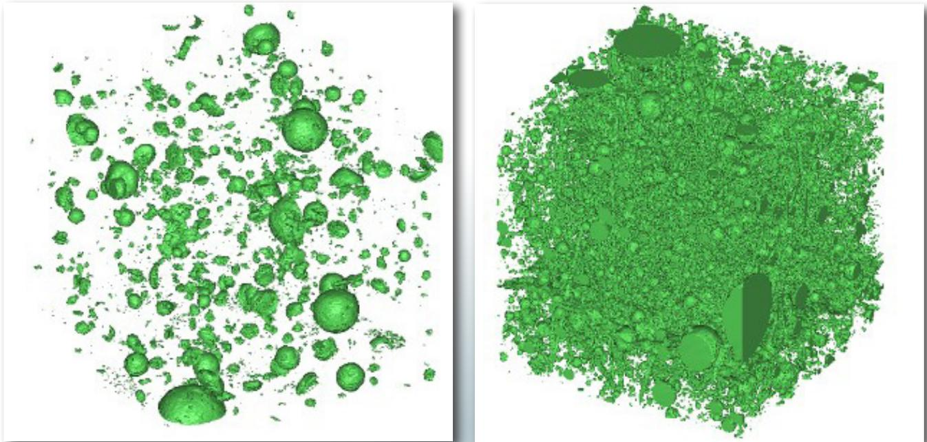
**Figure 2: Reconstructed 3D images of pore structure (in green color) for UHPC (left) and conventional concrete (right)**
