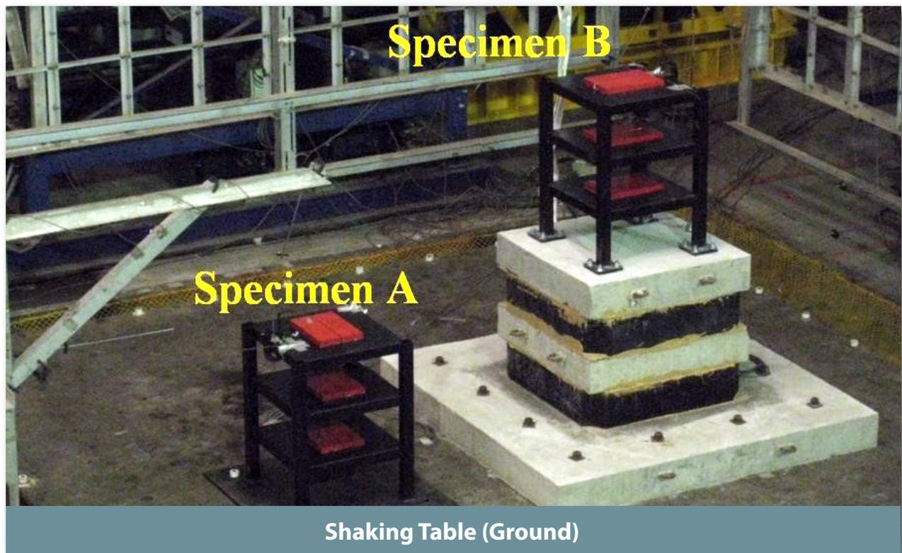
Figure 1: Test setup of 1D periodic foundation
