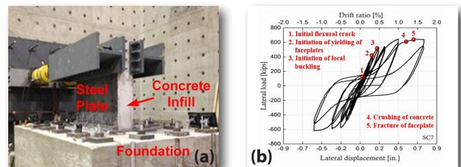
Figure 6: In-plane shear test – (a) test setup and (b) applied force – displacement response
