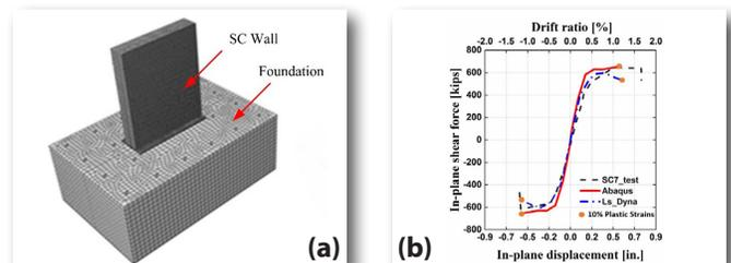
Figure 7: (a) In-plane shear analytical model test and (b) Analytically predicted response
