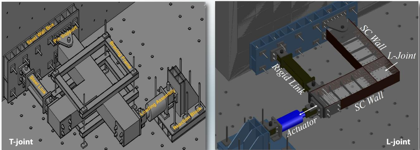
Figure 2: SC wall to wall connection test setup
