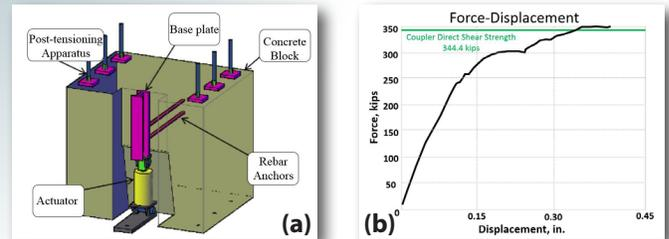
Figure 5: Direct shear test – (a) test setup and (b) applied force – displacement response
