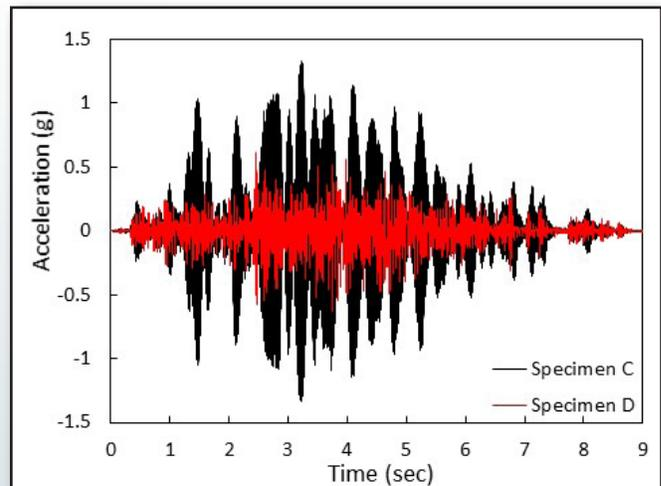
Figure 5: Test results of 2D periodic foundation
