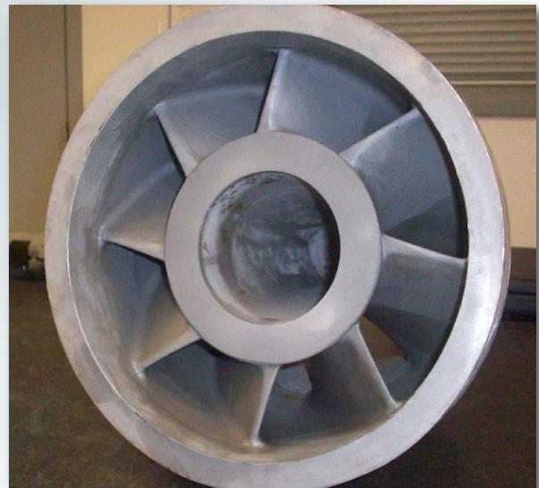
Figure 2: ALWR steam separator inlet swirler.
