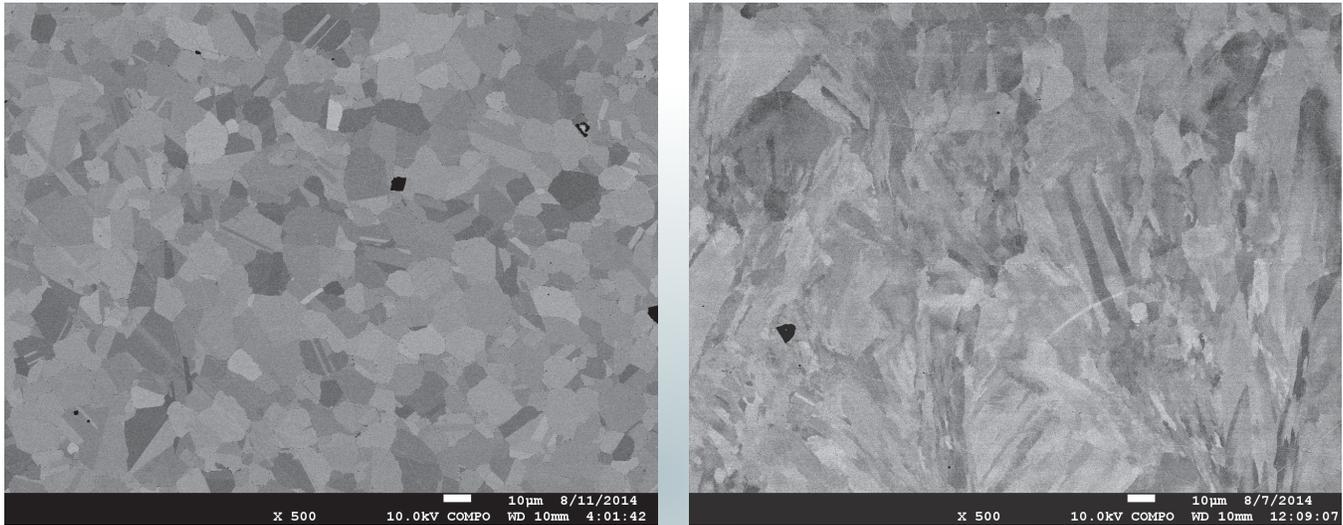
**Figure 4: Micrographs showing microstructure/grain size between Inconel bar stock (left) and additively manufactured sample (right).**
