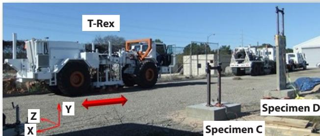
Figure 3: Test setup of 2D periodic foundation
