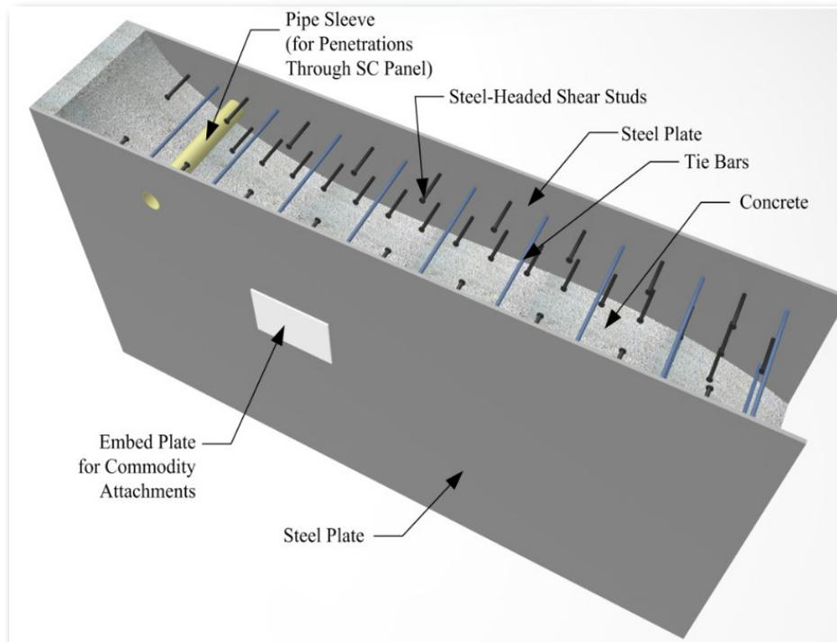
**Figure 1: Typical SC wall and its components**
