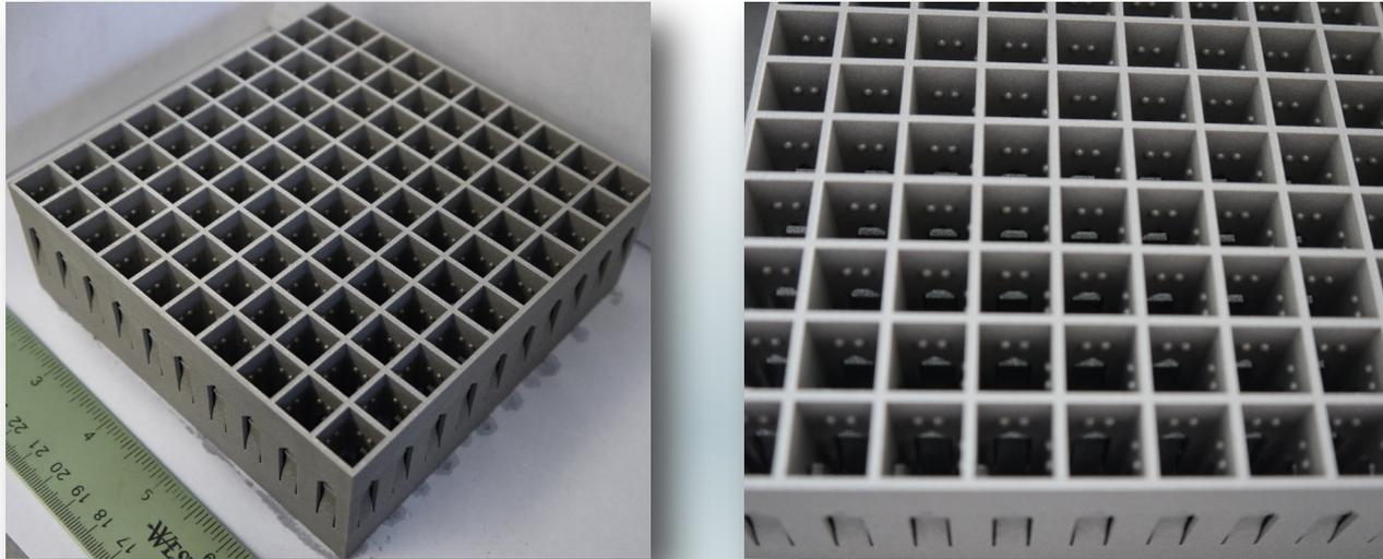
**Figure 2. Inconel 600 10x10 fuel rod spacer grids fabricated using DMLS demonstrating the structural detail that can be achieved**
