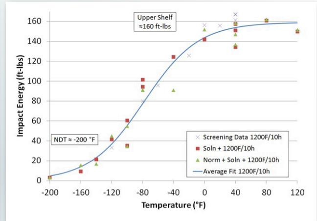
Figure 4. Charpy impact toughness results recorded for the SA508, Class 1, Grade 3 low hardenability test heat (Carbon equ.= 0.55).
