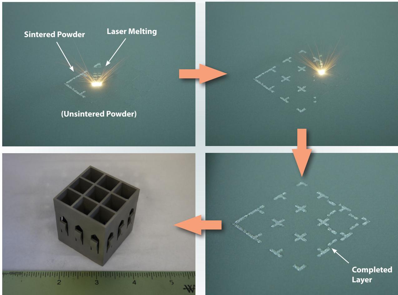
Figure 1. The sequence of steps in the layered build of a 316SSL demonstration article using DMLS
