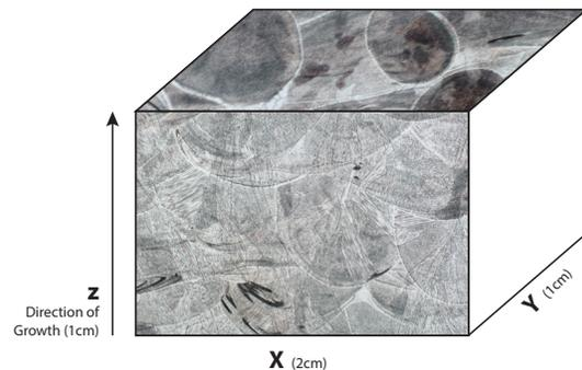
**Figure 3: Micrographs in the x-z and x-y planes for the quench melt puddle in an Inconel 600 sample.**
