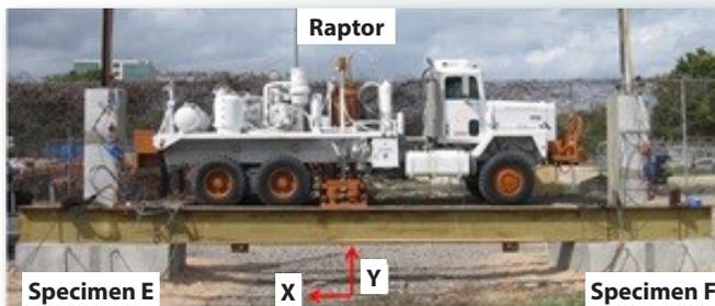
Figure 4: Test setup of 3D periodic foundation
