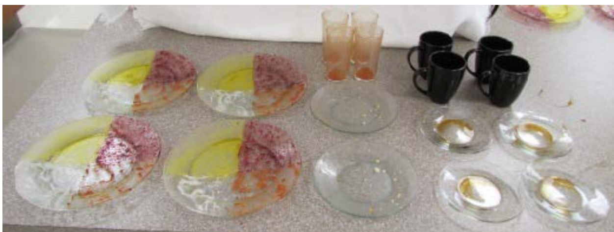
Figure 1—DOE (AHAM DW-1) Soil Using Clear Plates
