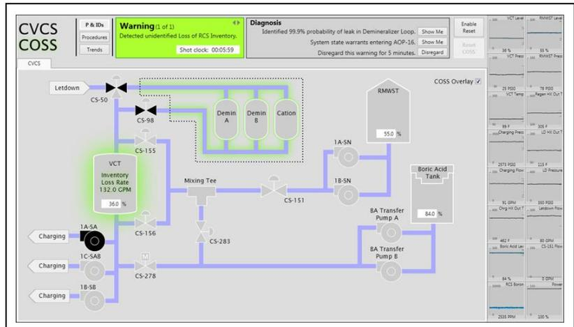
**Figure - COSS display featuring suggested mitigation actions and components related to the fault and the mitigation of the fault.**
