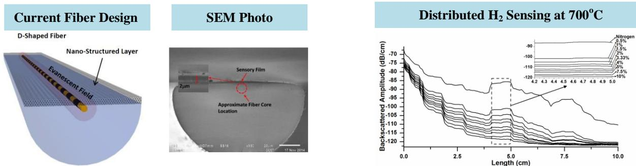
**Figure** - D-shaped fiber used for distributed hydrogen measurement and the results of hydrogen concentration measurement from 0.5% to 10% with 5-mm spatial resolution at 700°C.
