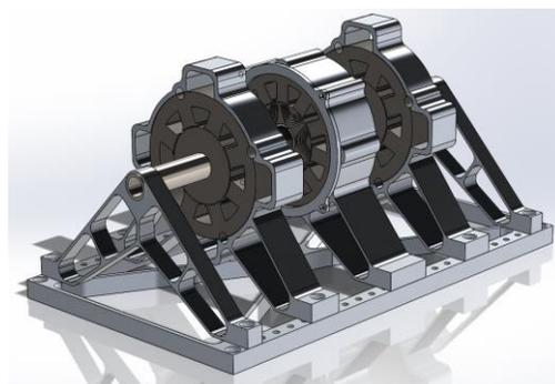
**Figure** - Test bed includes magnetic suspension bearings and main rotor drive.
