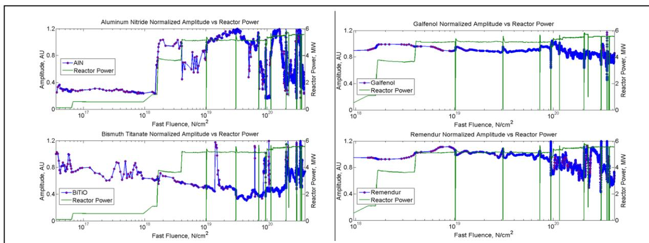
**Figure** - Signal amplitude of transducers as a function of total fluence. Bismuth Titanate transducer has degraded, as expected. Other transducers continue to operate with minimal radiation induced degradation.
