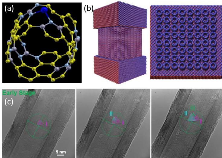
**Fig. 1** - (a) DFT simulation of  $BC_4N$  nanotube with Li. (b) MD model of BNNTs for simulating displacement cascade. An  $8 \times 8$  array of BNNTs is sandwiched by two cubic boron nitride substrates. (c) Early-stage evolution of irradiation-induced vacancy defects in multi-walled BNNTs as observed through in-situ TEM.
