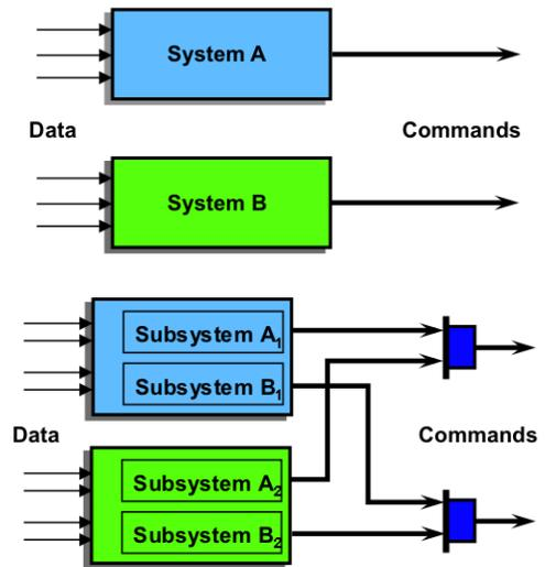
**Figure** - Typical safety system architectures for CCF mitigation: co-equal diverse systems (top) and functionally diverse subsystems (bottom).
