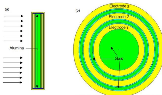
**Figure 1** - Conceptual model of fission chamber. (a) Longitudinal view. (b) Cross-sectional view.
