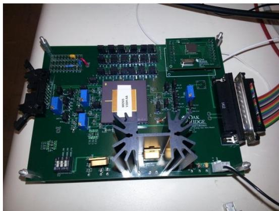
Figure - Board with radiation-hardened analog array.
