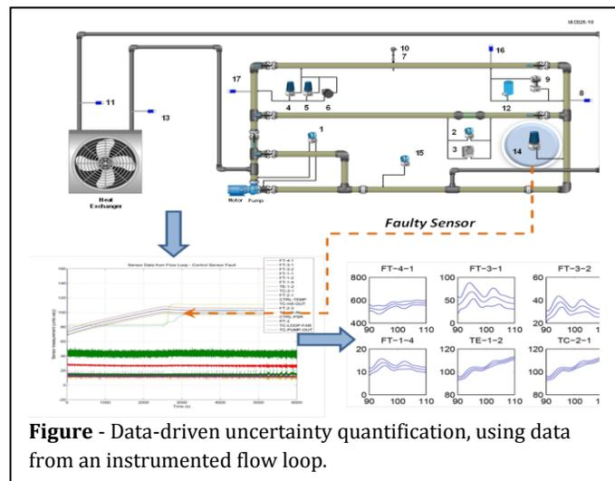
**Figure - Data-driven uncertainty quantification, using data from an instrumented flow loop.**
