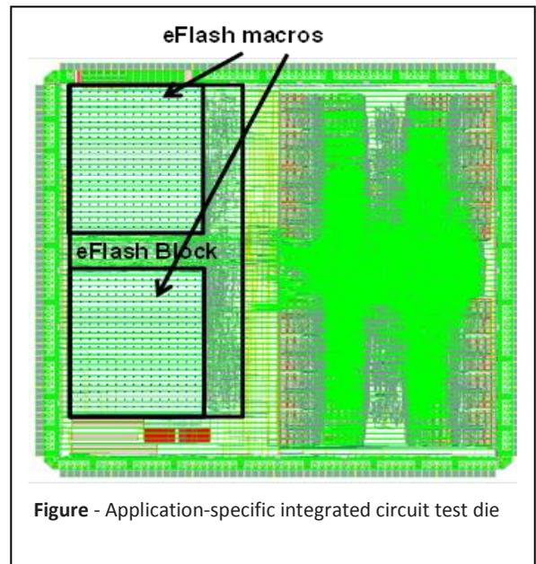
Figure - Application-specific integrated circuit test die
