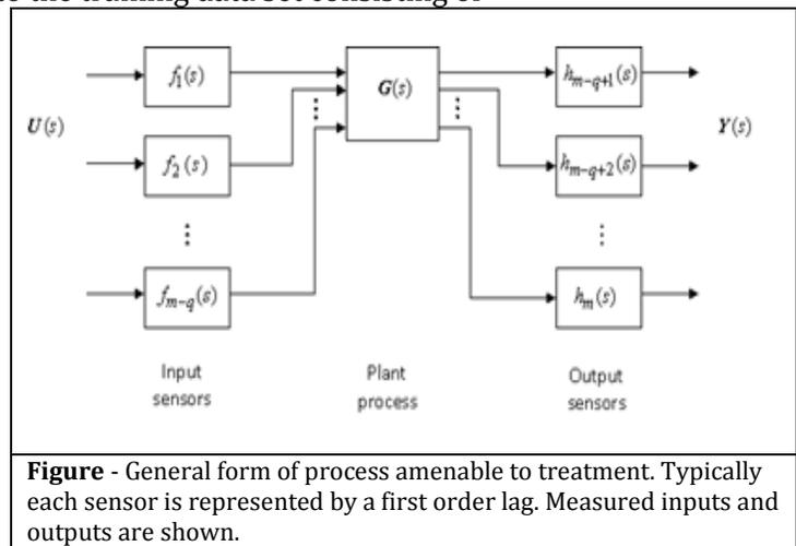
**Figure** - General form of process amenable to treatment. Typically each sensor is represented by a first order lag. Measured inputs and outputs are shown.
