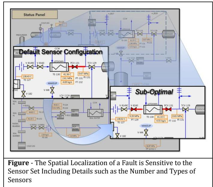
**Figure** - The Spatial Localization of a Fault is Sensitive to the Sensor Set Including Details such as the Number and Types of Sensors
