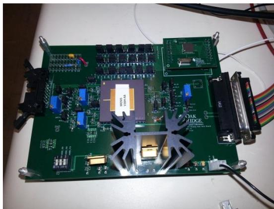
Figure - Board with radiation-hardened analog array.
