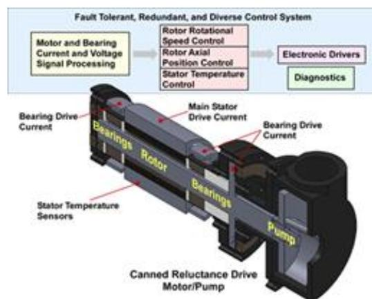
**Figure** - Fault-tolerant, redundant, and diverse control embedded in coolant circulation pump
