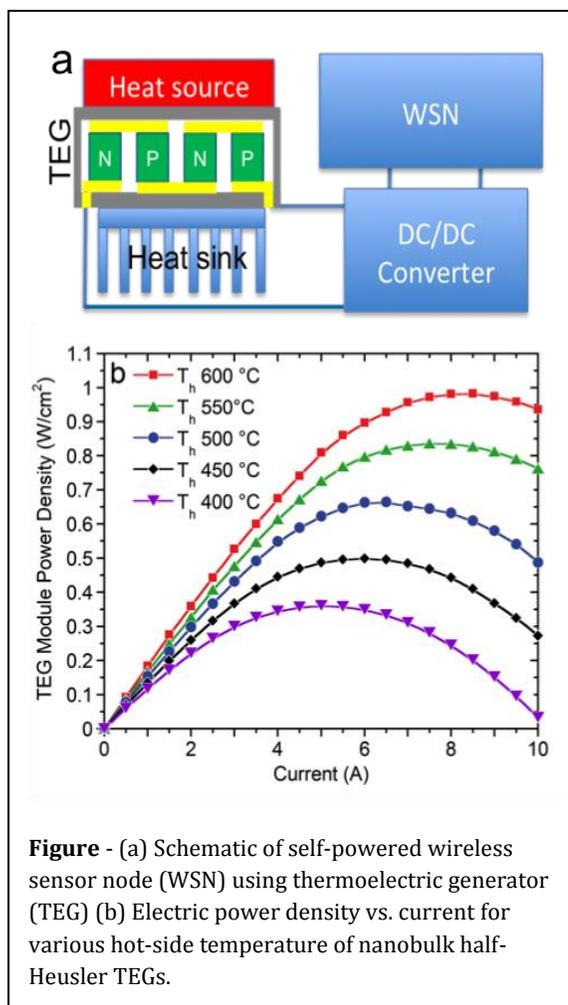
**Figure -** (a) Schematic of self-powered wireless sensor node (WSN) using thermoelectric generator (TEG) (b) Electric power density vs. current for various hot-side temperature of nanobulk half-Heusler TEGs.
