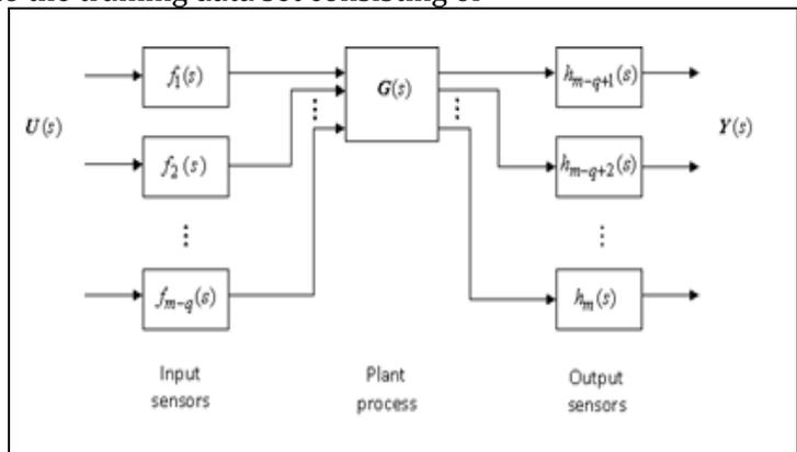
**Figure** - General form of process amenable to treatment. Typically each sensor is represented by a first order lag. Measured inputs and outputs are shown.
