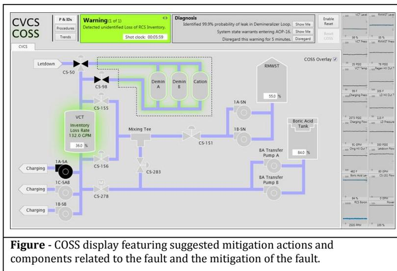
**Figure - COSS display featuring suggested mitigation actions and components related to the fault and the mitigation of the fault.**
