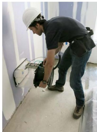
A powered-flow hood device is used to measure point-source leakage from an electrical outlet.
