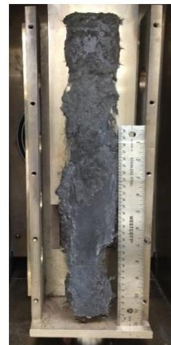
Figure IV-39: Sliding plate rheometer with a sample.
