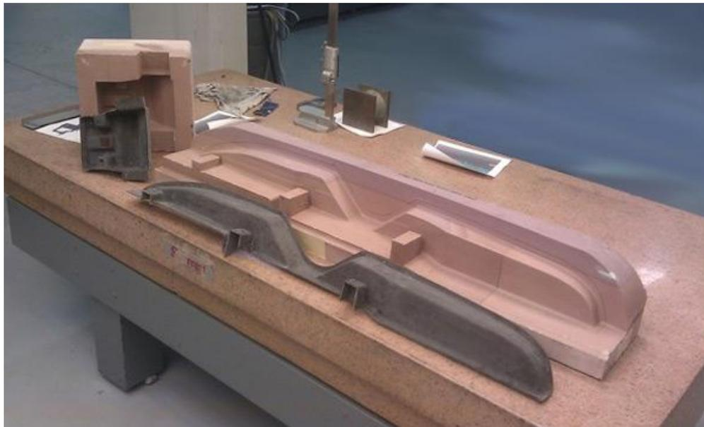
Figure V-19: CF Upper Duct and Plenum Bracket Parts and Tools.
