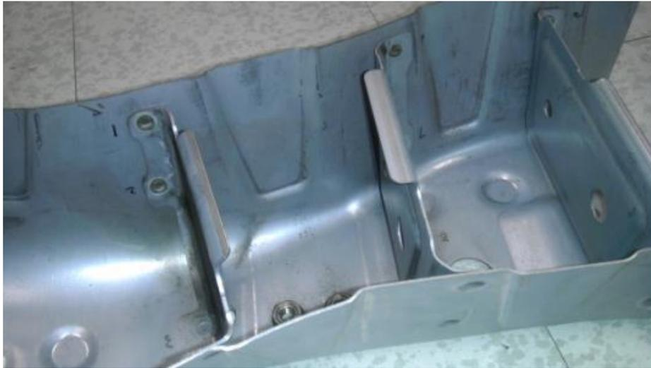
Figure III-71: Production auto body components with multiple spot welds used in field trials.
