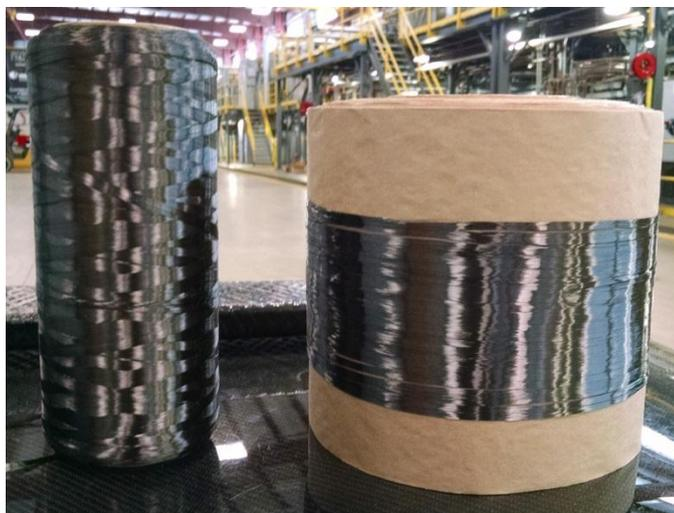
Figure IV-11: Typical spools of (a) 24 K industrial-grade carbon fiber and (b) 610 K rolls of textile-based carbon fiber.
