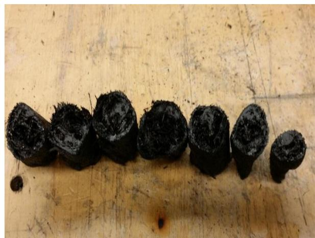
Figure IV-32: Nonuniform profile and voids within ASPN purges.
