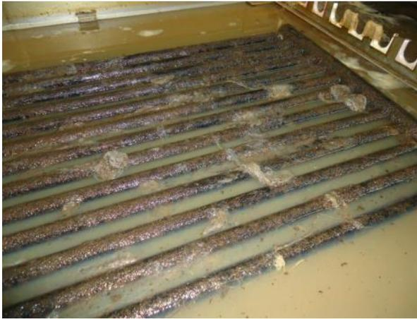
Figure IV-1: Heater coil in pre-stretching bath saturated with non-soluble residue during commercial spinning trial
