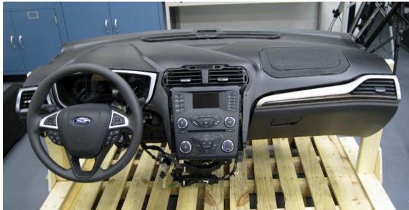
Figure V-21: Complete Carbon Composite MMLV IP/CCB.
