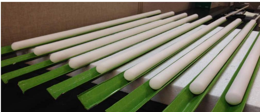
Figure III-16: Fired zirconia tubes for electrolysis tests.
