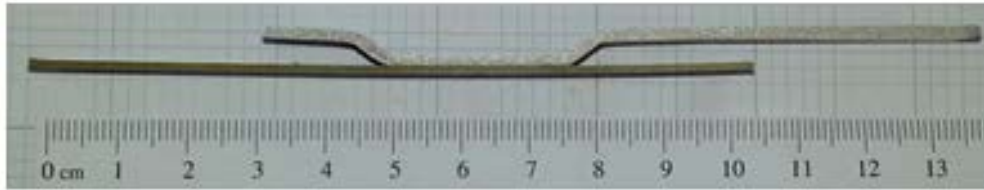
2mm thick Al6061-T4 welded to DP780 steel
