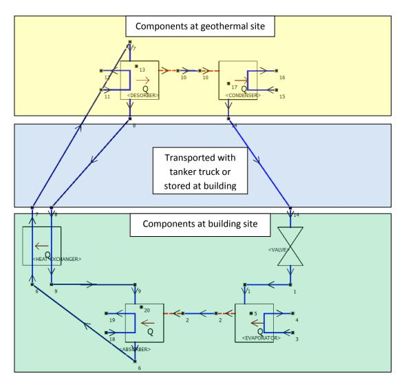
Determined design parameters for proposed system based on simulation results using ORNL's SorpSim program
