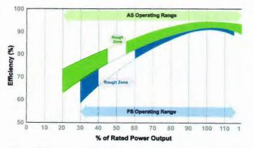
Figure 2. Comparison of Efficiency Curves in Generation Mode for FS (Blue) and AS (Green) PSH Units (adapted from USACE 2009<sup>6</sup>).
