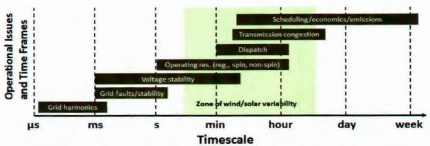
Figure 3. Overview of Issues in Power System Operations and Control (adapted from Fisher et al. 2012<sup>8</sup>).
