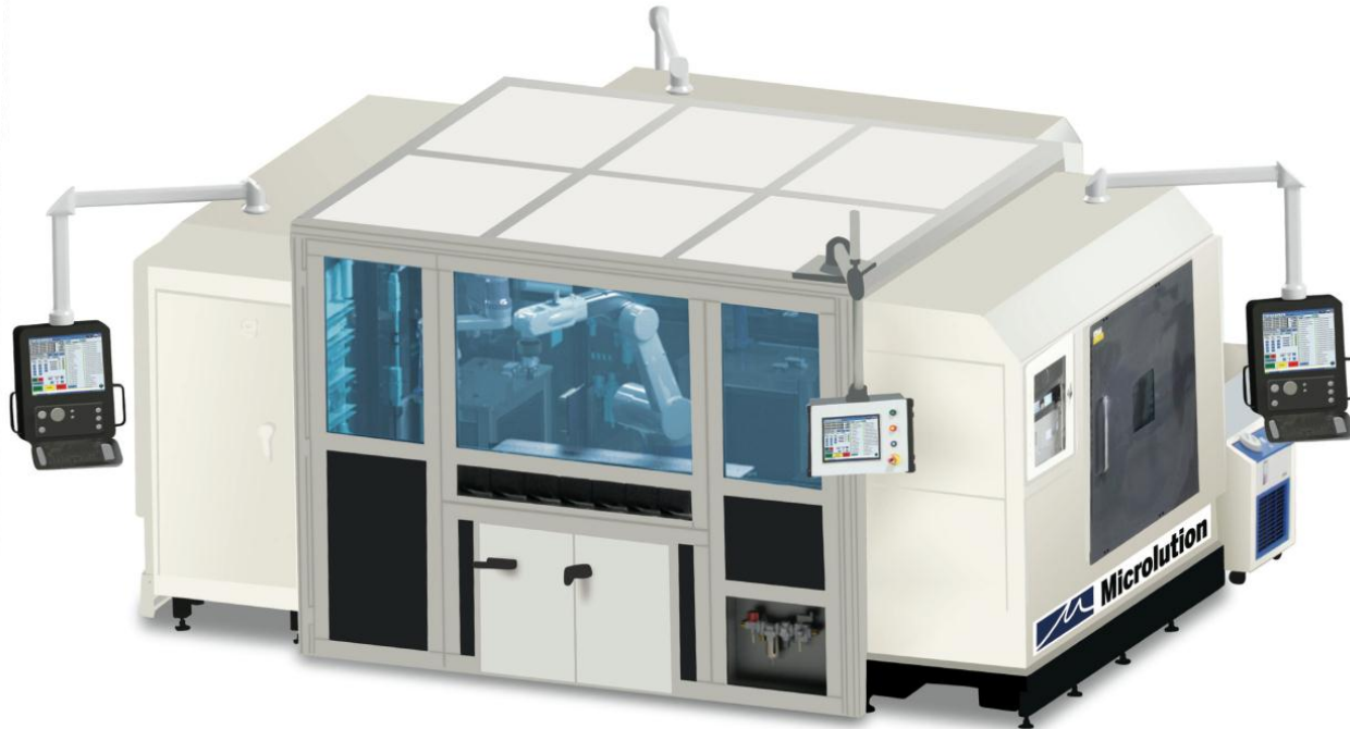
Example of First-Generation Laser Cell Installed for Biomed Mfg
