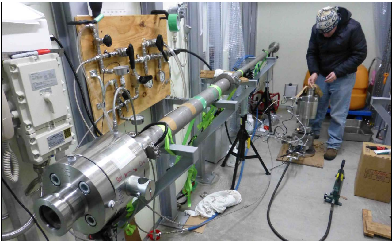
Figure 1: In January, 2013, scientists from AIST, JOGMEC, Georgia Tech, and the USGS collaborated in the analysis of pressure cores of gas hydrate-bearing sand reservoirs collected offshore southeastern Japan using tools developed under the DOE Gulf of Mexico JIP. Photo courtesy USGS.
