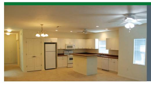
One-fourth of the homes' lighting fixtures are LED-based; the remaining lights are compact fluorescent. ENERGY STAR dishwashers and refrigerators further reduce energy use. Each home has five ENERGY STAR-rated ceiling fans to help reduce the need for air conditioning.
