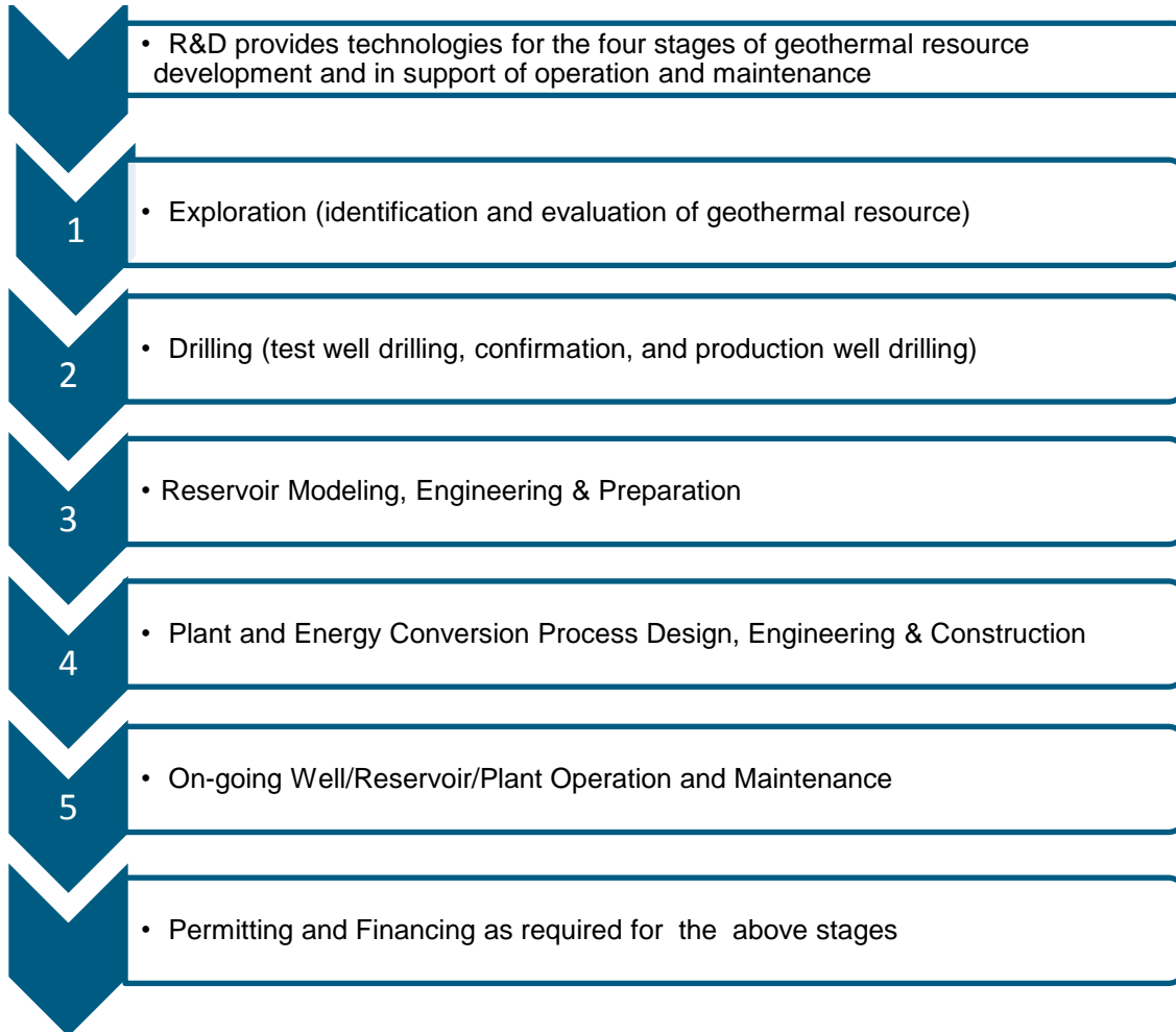
Figure 2-1. Activities in Developing Geothermal Energy Power Generation, and Supporting Functions
