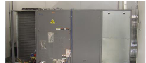
UTRC CCCHP Prototype System
