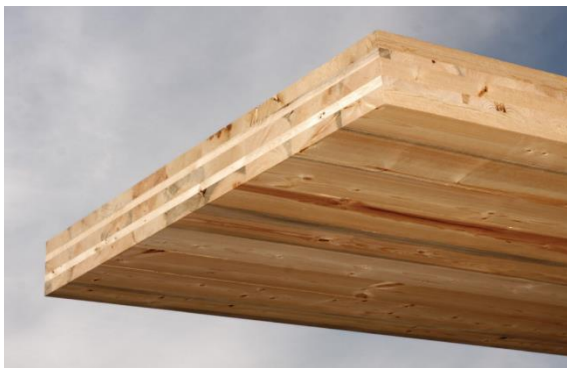
Figure 18 - A Close-up of the CLT Slab (CST Innovations, 2015)
