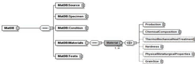
Figure 1. Hierarchical structure of the MatDB.
