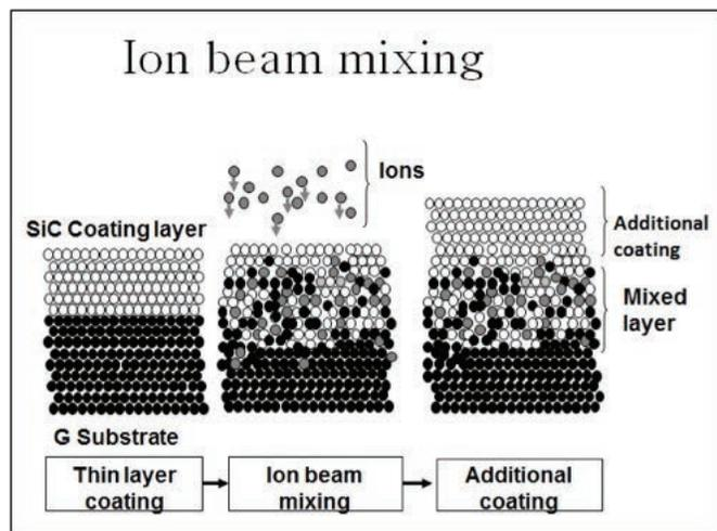
Figure 2. Schematic illustrating the ion beam mixing processes.
