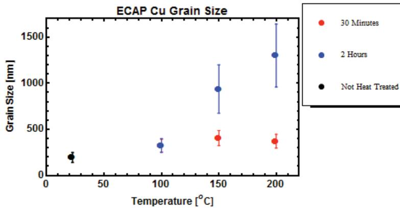
Figure 1: Grain size as a function of heat treatment measured using Scanning electron Microscopy and the intersect methods.
