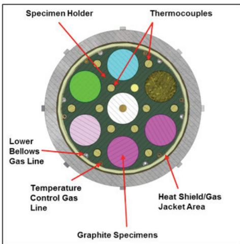
Figure 7. AGC irradiation test train cross-section illustrating specimen columns. Six outer columns are tested under a mechanical load while the central column is unloaded. SiC coated specimens will be irradiated in the central unloaded column.
