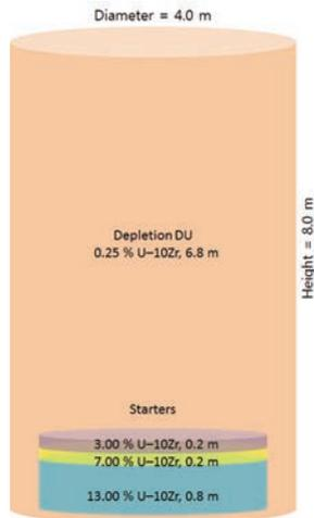
Figure 1. Conceptual Drawing of CANDLE Core
