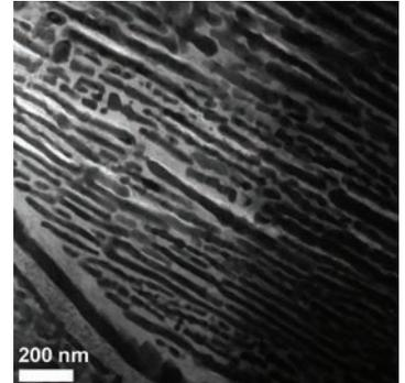
Figure 3. TEM micrograph obtained from an as-cast 52U-20Pu-3Am-2Np-8.0Ln-15Zr sample showing nano-sized light and dark contrast grain structure.
