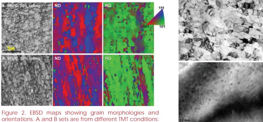
Figure 2. EBSD maps showing grain morphologies and orientations. A and B sets are from different TMT conditions: 900°C 20% rolling and 975°C 50% rolling, respectively
