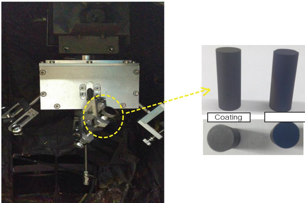
Figure 4. Image of rotating jig inside the coating/ion mixing chamber. The 360° rotation allows uniform coating of entire specimen.
