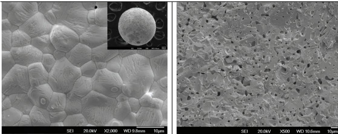
Fig. 2. Scanning electron microscopy of UCN kernels showing kernel surface (left image) and kernel interior (right image).
