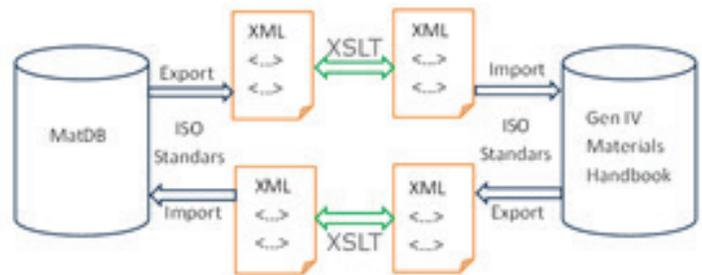
Figure 6. Achieving interoperability for massive digital data exchange.
