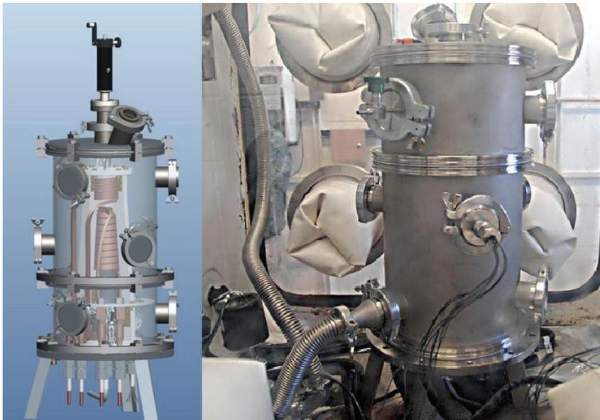
Figure 2. Schematic and photo of GACS configured for gravity casting. Note the linear actuator has been removed for the photo.
