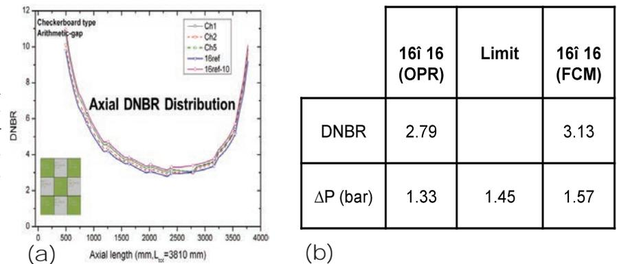
Figure 5. Mixed transition core compatibility analysis of (a) axial DNBR distribution and (b) standard and FCM DNBR and  $\Delta P$  results and limits.
