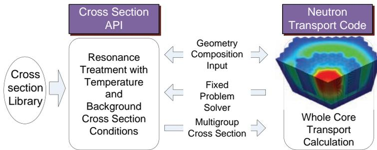
Figure 2. Interaction between Cross Section API and Neutron Transport Solver
