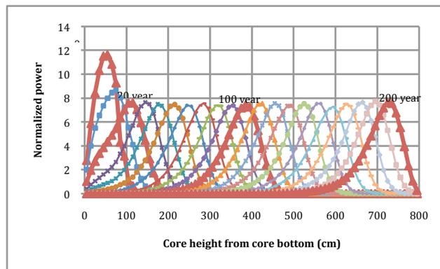
Figure 3. Propagation of Axial Power Profile in CANDLE
