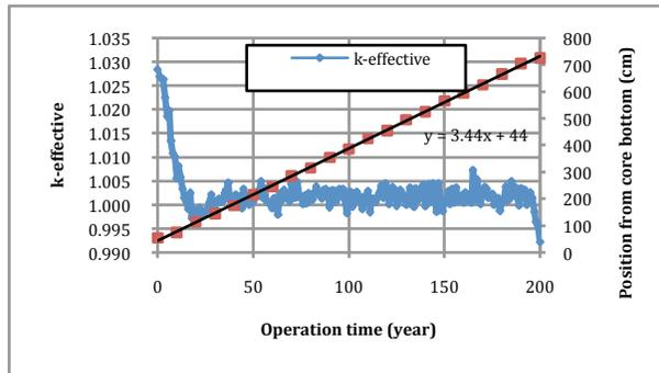
Figure 2. Feasibility Test of Breed-and-burn Core Concept with CANDLE Model
