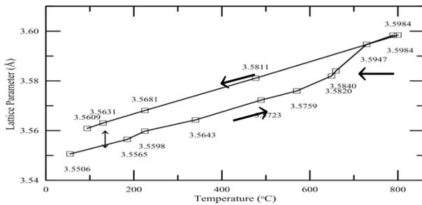
Figure 3: Lattice parameter as a function of temperature for a Ni<sub>2</sub>Cr sample initially aged for 8,000h at 475°C. This was conducted at the Advanced Photon Source (APS) at (ANL).
