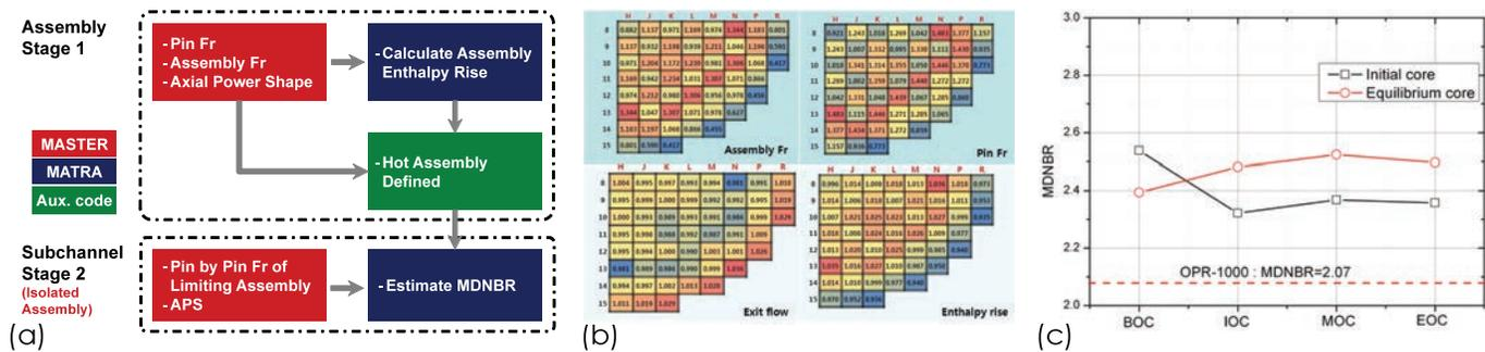
Figure 6. Core TH assessment (a) two-step method used for margin analysis, (b) quarter-core power distributions used for TH calculations, and (c) MDNBRs calculated for transition cores fully loaded with 16x16 FCM FAs
