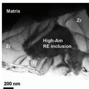
Figure 5. Left: high Am content RE inclusion surrounded by high Zr content inclusion.
