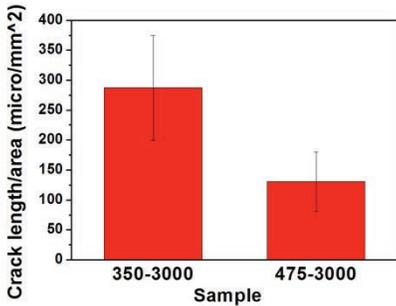
Figure 6: Crack counting results of cold rolled and thermally treated samples with two aging conditions which were strained to 2% at  $1 \times 10^{-8}$  s<sup>-1</sup> in 360 °C water containing 18 cc/kg H<sub>2</sub>.
