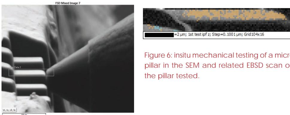
Figure 6: insitu mechanical testing of a micro pillar in the SEM and related EBSD scan of the pillar tested.
