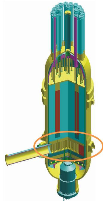
Figure 1. Schematic of a VHTR design illustration the core support region.
