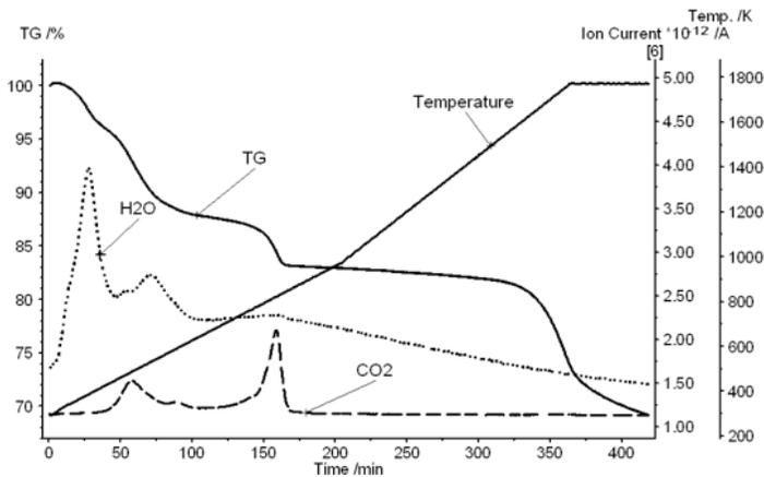
Fig. 1. Characteristics of calcination of air-dried UO<sub>3</sub>:2.65C in argon from thermogravimetry and mass spectrometry.
