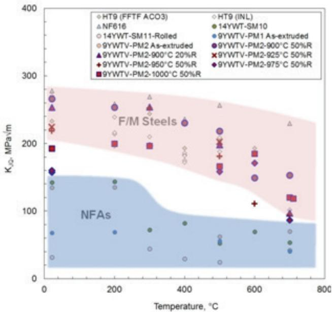
Figure 4. Fracture toughness data of 9YWTV-PM2 after hot-rolling at 900°C, 925°C, 950°C, 975°C, and 1000°C, compared to the data for FM steels and other NFAs.
