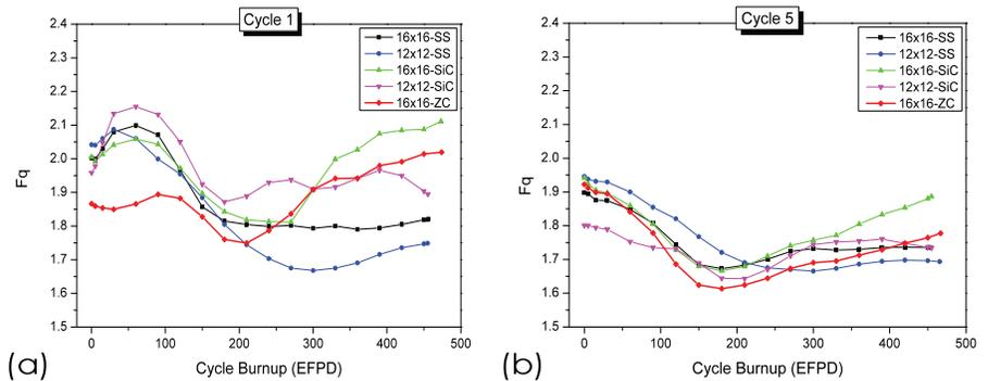
Figure 3. Power peaking factors for OPR-1000 FCM replacement fuels in (a) Cycle 1 and (b) Cycle 5 (equilibrium cycle).
