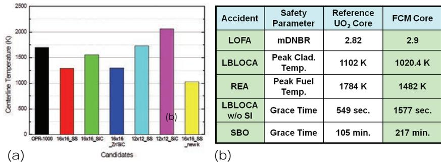
Figure 7. (a) Results from initial stored energy analyses and (b) enhanced accident tolerance for 16x16-ZC FCM FAs for limiting DBAs and BDBAs.
