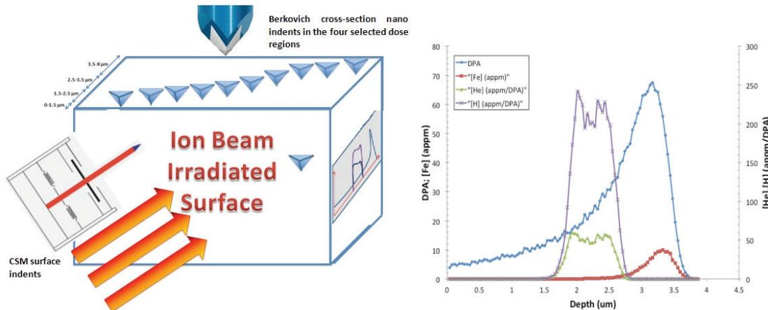
Figure 4: Sheamtic sketch of the mechncail testing vs. ion beam irradiation profile on the tripple ion beam irradiated samples.
