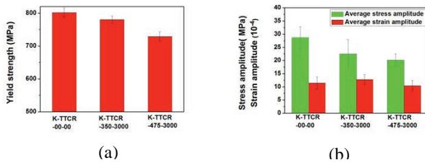
Figure 5: (a) Yield strengths and (b) average stress and strain amplitudes of serrations of thermally treated and cold-rolled samples in the un-aged and aged conditions which were strained in 360 °C water containing 18 cc/kg H<sub>2</sub>
