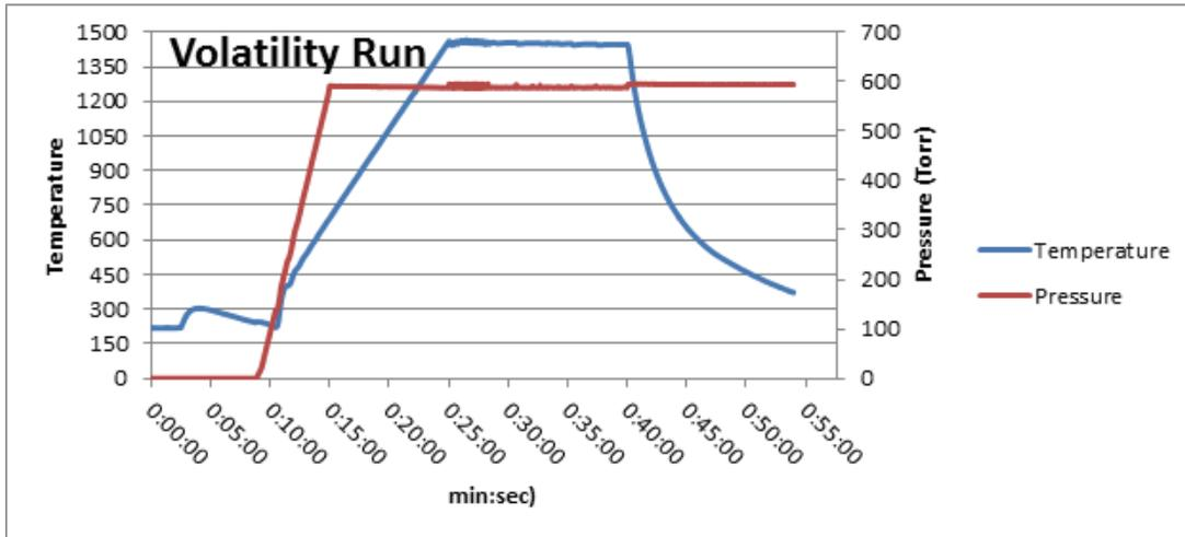
Figure 4. Typical furnace pressure and temperature profile for the volatility experiments.
