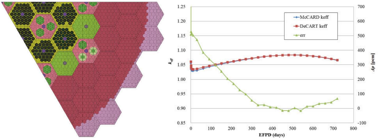
Figure 1. DeCART 2D 1/6 Core Model and Depletion Calculation Results for HTR
