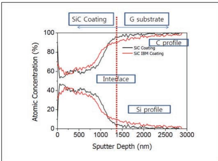
Figure 6. Auger analysis of initial SiC coating. The coating with IBM shows more broadened interface than a coated interface without ion beam mixing. Analysis illustrates functionally gradient coating resulting from IBM.
