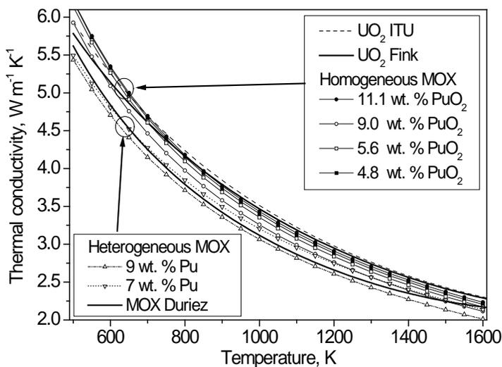
Figure 6. Experimental thermal conductivity of homogeneous and heterogeneous MOX compared to UO<sub>2</sub> (95 %TD) [from Staicu & Barker, 2013].
