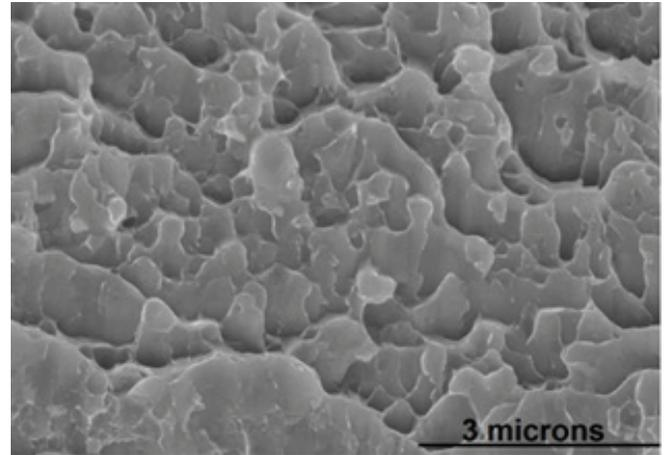
Figure 5. Fracture surface of 9YWTV-PM2 tested at 700°C after 50% hot-rolling at 900°C.
