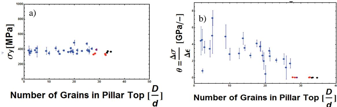
Figure 2: Yield stress as a function of pillar diameter to grain size ratio of the as processed sample with 200nm grain size. The black and red dots are the data points measured by macroscopic tensile testing. It is found that no change in yield stress is observed a). Work hardening as a function of pillar diameter to grain size ratio. A decrease in work hardening can be observed with sample size.
