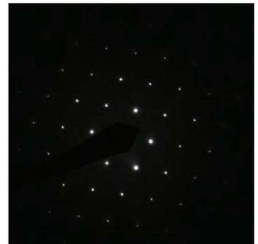
Figure 4. Electron diffraction pattern from a Zr rich inclusion along the [110] axis revealing it to be in the, to date, unreported face-centered-cubic structure.
