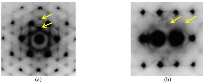
Figure 1: Typical selected area diffraction patterns (SADPs) from Alloy 690 showing diffuse scattering at the  $\{422\}$  positions in the  $\langle 111 \rangle$  pattern (a) and the  $\frac{1}{2}\{311\}$  in the  $\langle 112 \rangle$  pattern (b).
