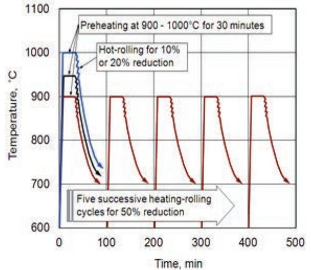
Figure 1. Schematics of controlled rolling (CR) treatments applied to Fe-9Cr base NFAs.
