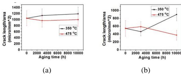
Figure 4: Crack length per unit area of (a) solution annealed and aged samples, and (b) thermally treated and aged samples which were strained to 7% at  $5 \times 10^{-8}$  s<sup>-1</sup> in 360°C water containing 18 cc/kg H<sub>2</sub>.
