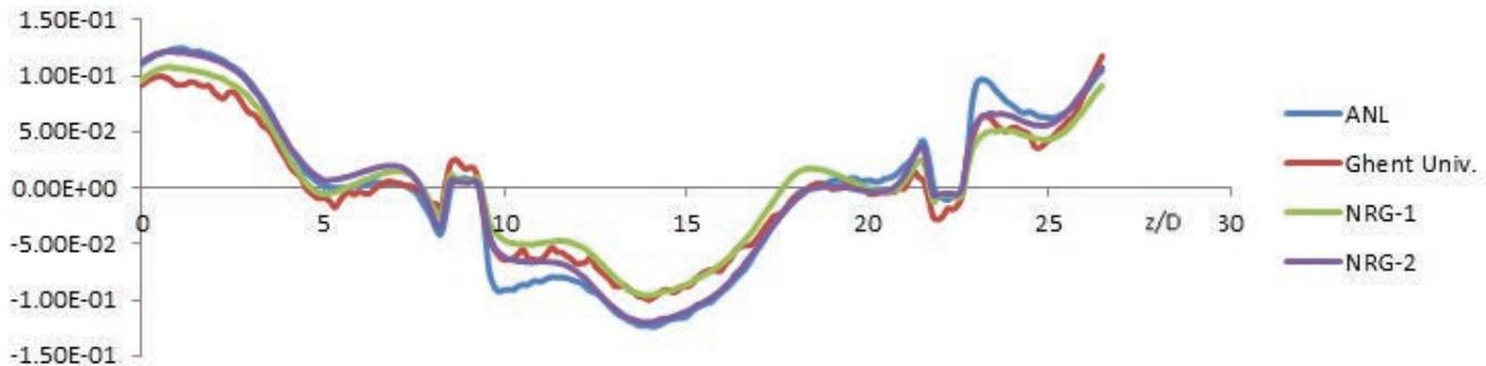
FIGURE 1. One of the cross flow comparisons in the 7 pin rod bundle benchmark – Central pin. Cross flows are normalized by  $U_{bulk} \cdot g$  (where  $g$  is the gap size without wire).
