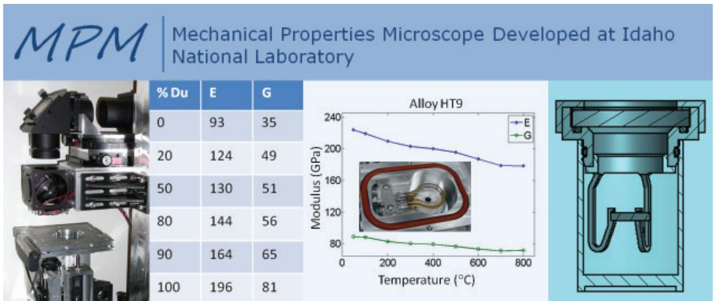
Figure 7. Left: Photograph of MPM, Left-middle: Elastic constants of UZr system vs. composition (values reported in GPa), Right-middle: Elastic constants of HT9 vs. temperature (inset: heating furnace), Right: Sample loading capsule.
