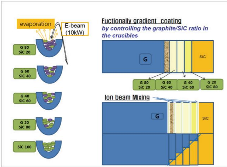
Figure 5. Schematic of E-beam evaporative coating deposition process. A functionally graded coating is created by melting and depositing successive layers with different compositions of materials as illustrated by the different materials on the left side of the graphic. Ion beam mixing is used between successive deposits to create a gradual gradient rather than a step-wise gradient of material compositions.
