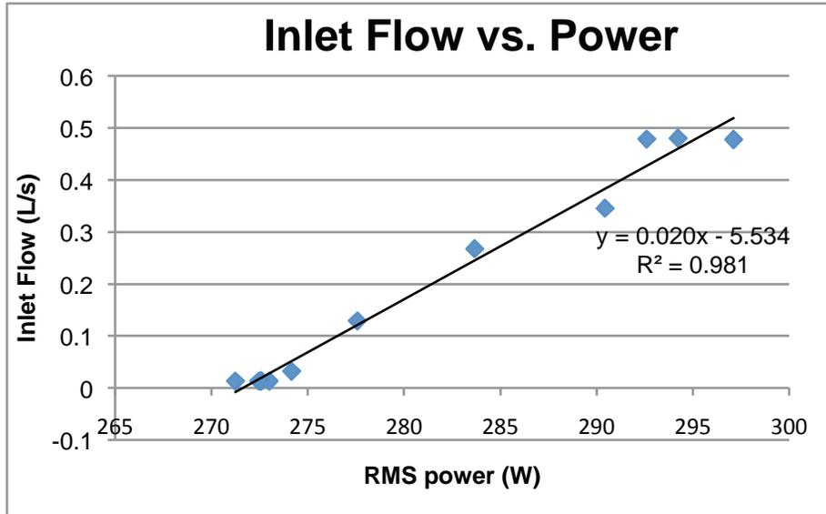
Figure 7. The RMS power drawn by the pump increases as the flow rate increases
