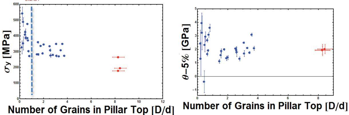
Figure 3: Yield strength as a function of the ratio of pillar diameter vs. grain size. It can be seen that these samples do show a size effect. Again the red data points are the tensile test data. B) work hardening as a function of the ratio of pillar diameter vs. grain size.
