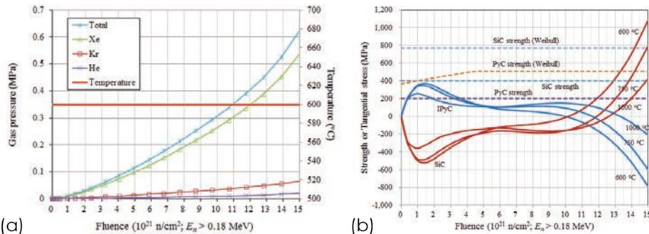
Figure 7. (a) Fission gas pressure in TRISO at 850°C and (b) stress at TRISO layers at 850°C.
