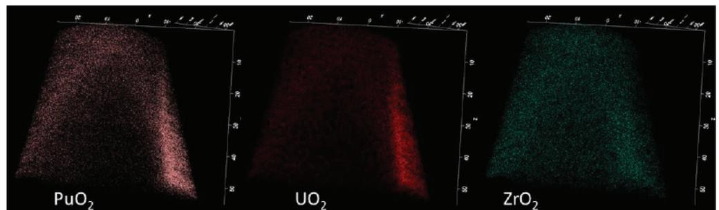
Figure 2. Reconstruction of U-55Pu-20Zr samples showing the Pu/U rich and Zr depleted region at the edge of the samples that is hypothesized to be a former grain boundary region.
