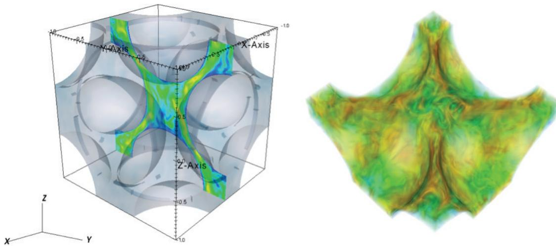
FIGURE 2. Pebble bed simulations at Argonne. (left) View of the computational domain and cross section with snapshot of the instantaneous velocity magnitude (right) volume rendering of the velocity field.
