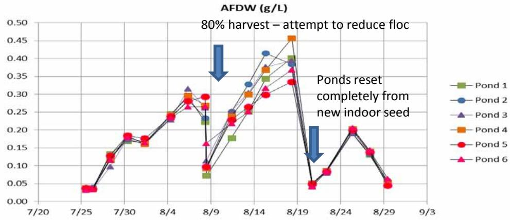
Suboptimal pond performance as indicated by AFDW and O.D. and physical observation - ponds flocculating
