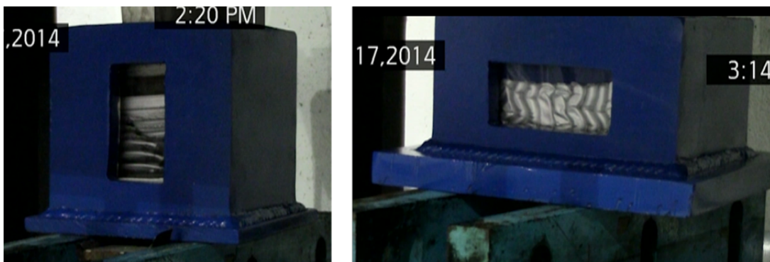
Figure III - 31: Photographs of batteries in the sleeve constraint for mechanical testing in the end and side orientations
