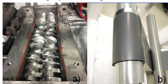
Figure II - 6: a) Inline mixer b) Calendared electrode (inline mixed)
