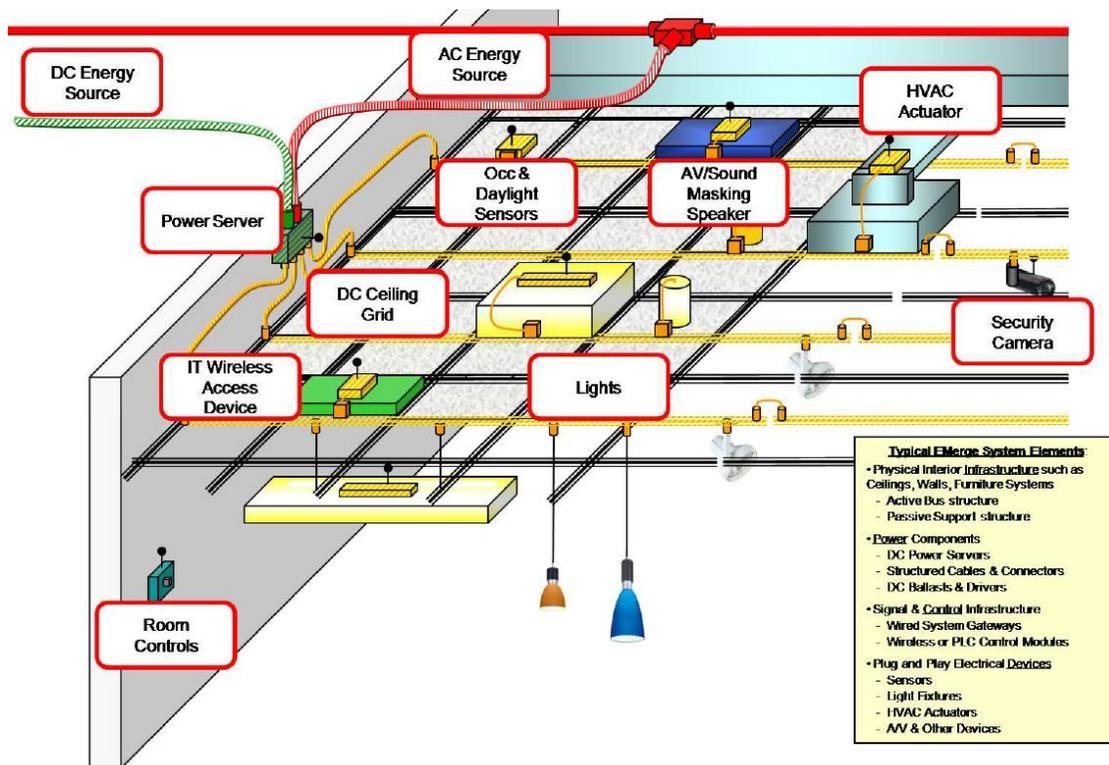
Figure 6. Ceiling DC distribution system architecture block diagram [4].
