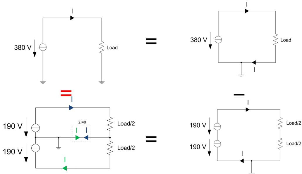
Figure 11: Investigation of  $\pm 190\text{Vdc}$  topology in comparison with the  $+380/0\text{ Vdc}$  topology
