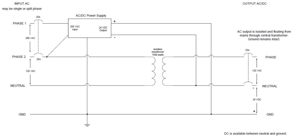
Figure 1. Hybrid AC/DC distribution option proposed by Nextek [2].
