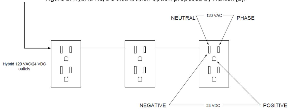
Figure 2. Wall outlet port configuration of the Nextek hybrid AC/DC distribution system.
