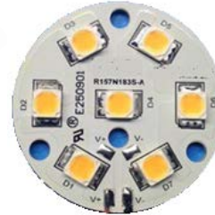
3020 PCT/3030 EMC light-engine
