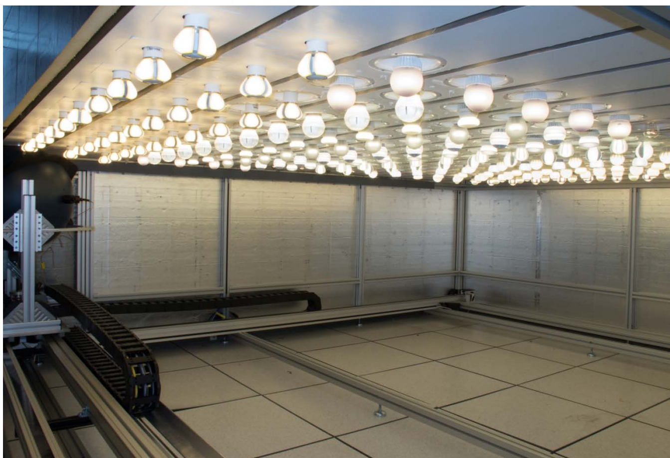
Figure 1. The ALTA apparatus with 170 A lamps from CALiPER Retail Lamps Study 3 (right) and 34 L Prize lamps (left) installed. The lamps protruded approximately 2" into the space below the mounting channels.
