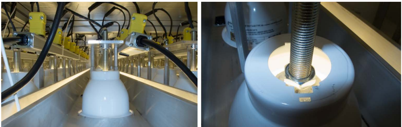
Figure 2. Reflector cones used to isolate individual lamps for measurement. The lamps were not completely sealed off, allowing for a minimal amount of spill light to reach the integrating sphere.
