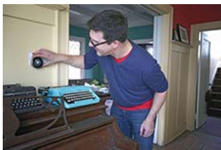
Marshall Runkel adjusts the Nest Learning Thermostat that optimizes the energy upgrades he is making to his North Portland home. Photo: Jonathan House
