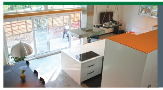
Large south-facing triple-pane windows keep out the cold while allowing in any available sunlight to warm the stainedconcrete thermal mass of the main floor. Radiant heating loops with hot water from an air-to-water heat pump provide radiant heat to the home. ENERGY STAR appliances, an induction cooktop, and 100% LED lighting help to keep energy usage to a minimum.
