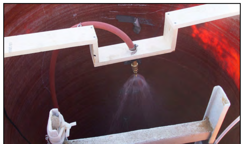
Figure 1. The first tests at the Mound system (left) used a small garden fountain pump attached to landscaping mist nozzles, with an air monitor to detect whether the contaminants were moving from the water to the air. The test was performed in a plastic box. The next test (right) used a larger pump and spray nozzle. Both showed that air stripping removed contaminants from the groundwater, and led to a larger air stripper at the Mound system (not shown).
