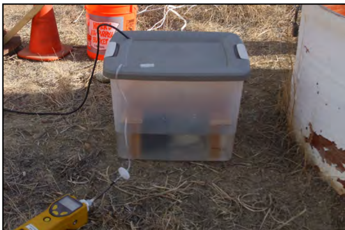
Figure 1. The first tests at the Mound system (left) used a small garden fountain pump attached to landscaping mist nozzles, with an air monitor to detect whether the contaminants were moving from the water to the air. The test was performed in a plastic box. The next test (right) used a larger pump and spray nozzle. Both showed that air stripping removed contaminants from the groundwater, and led to a larger air stripper at the Mound system (not shown).
