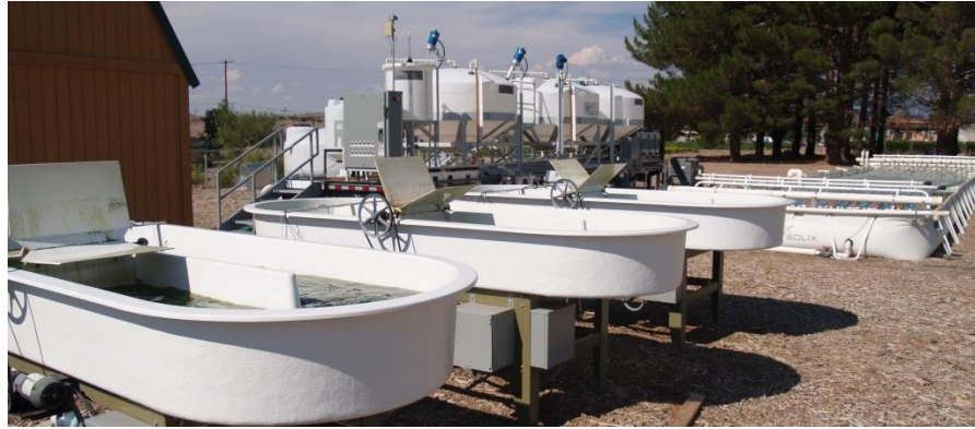
Raceways and Solix System - Centrifuge harvester
