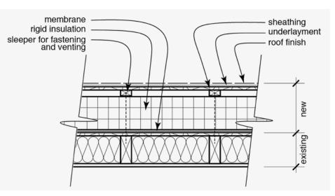
In the ETMMS process, a continuous air/water barrier is applied to the existing roof decking. Insulation is then added over the air barrier with seams staggered to reduce air leakage. Sleepers are placed between the insulation and new roof decking to create an air space for venting. The gable ends are addressed in a similar manner.
