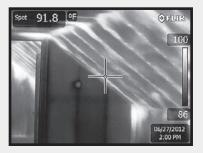
The light-colored areas of the infrared image taken before construction highlight air leakage and thermal bridging that can lead to heat loss, snow melt, and ice dam formation.
