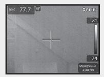
The infrared image taken after a roof-only ETMMS installation demonstrates the effectiveness of a continuous air barrier and insulation to reduce air leakage and thermal bridging at the roof level.
