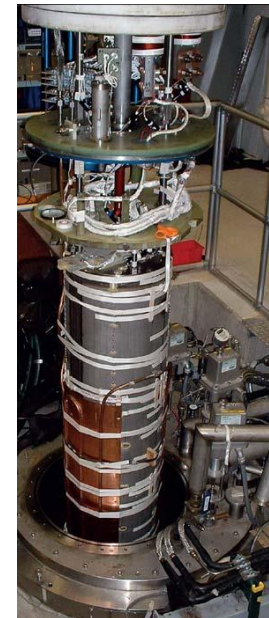
11 Tesla magnet test at Fermilab
