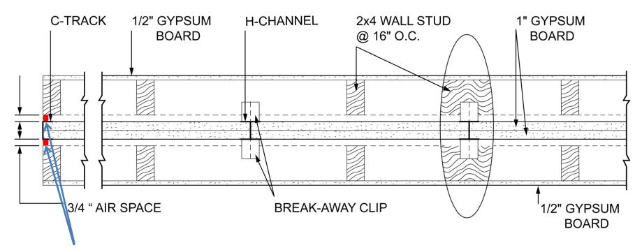
Fireblocking sealant to create air seal at perimeter of gap between area separation wall and protected wall.
