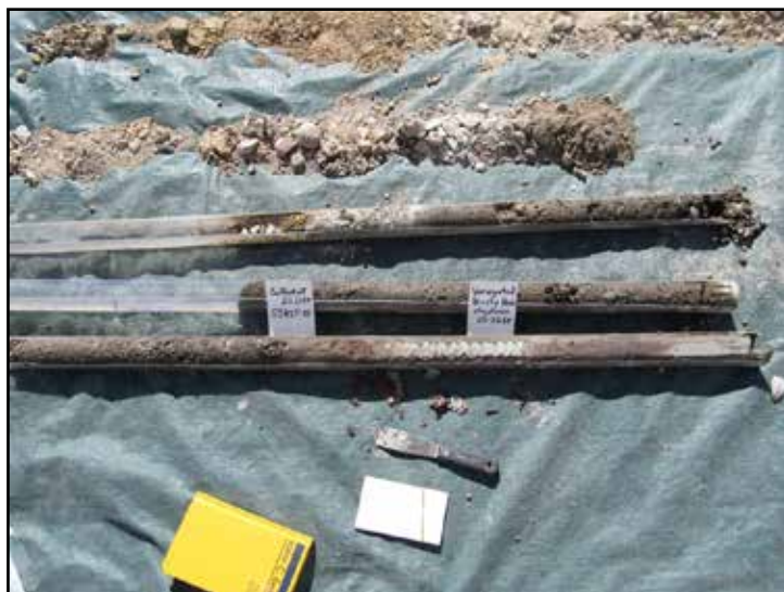
Core samples collected at the drill site are labeled with description information, placed in bags, and transported to a laboratory.
