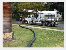
Hydrovac trucks have been used for decades. They can move 5,500 cfm of air and remove debris at 220 mph.
