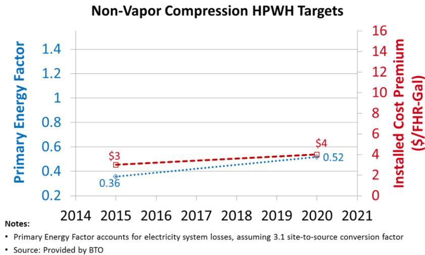
**Figure 1-6: Cost and Efficiency Targets for Non-Vapor Compression Technologies**
