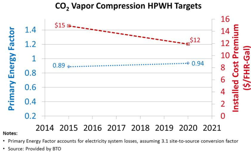
**Figure 1-5: Cost and Efficiency Targets for CO<sub>2</sub> Vapor Compression HPWH**
