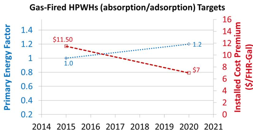
**Figure 1-7: Cost and Efficiency Targets for Gas-Fired HPWH**
