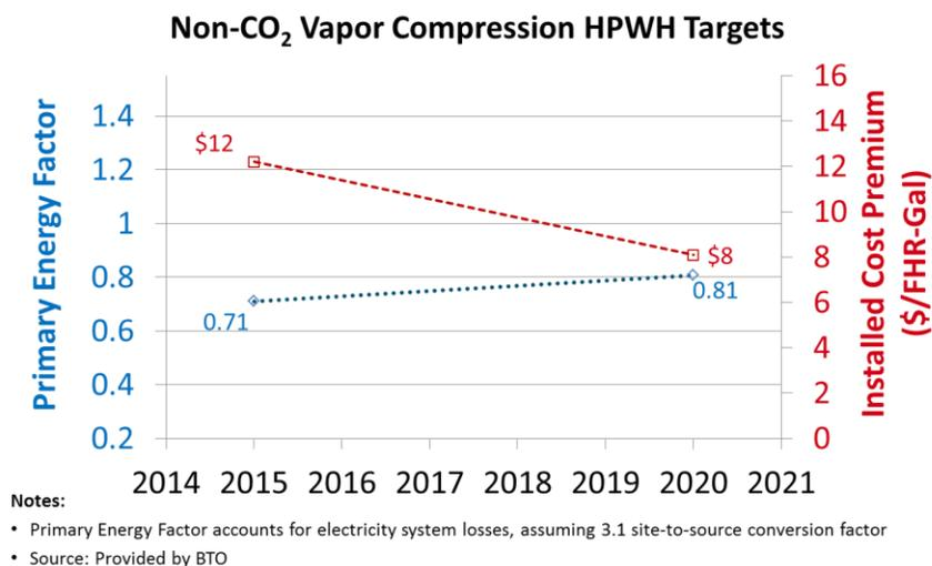
Figure 1-4: Cost and Efficiency Targets for Non-CO<sub>2</sub> Vapor Compression HPWH
