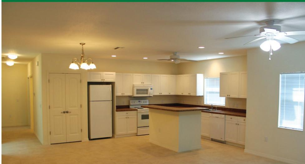
One-fourth of the homes' lighting fixtures are LED-based; the remaining lights are compact fluorescent. ENERGY STAR dishwashers and refrigerators further reduce energy use. Each home has five ENERGY STAR-rated ceiling fans to help reduce the need for air conditioning.
