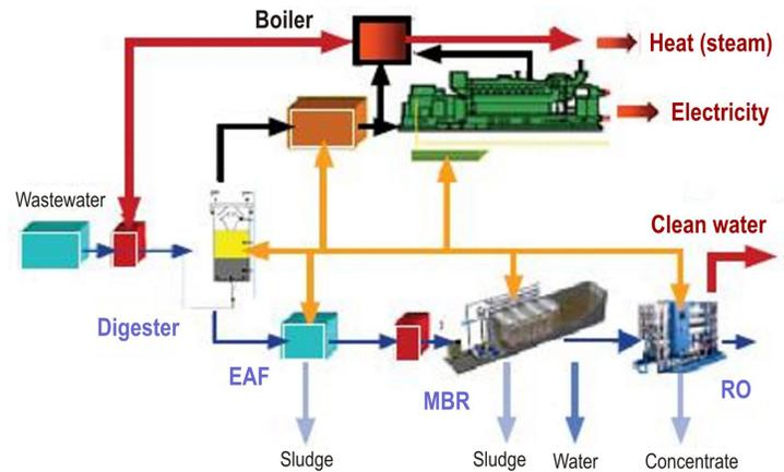
Waste-to-value plant recovers energy through anaerobic digestion and purifies the water to desired purity for reuse, moving through filtration, an aerobic membrane bioreactor (MBR), and reverse osmosis (RO). Predictive monitoring and supervisory controls are key to achieving the robust and flexible operation of the integrated plant. *Illustration courtesy of GE Global Research*
