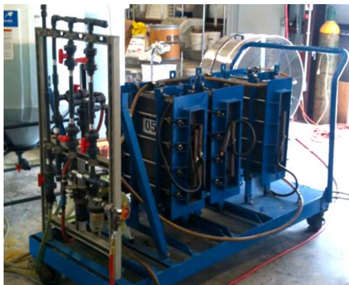
Figure 18. Kaselco reactor test bed at NAABB's Pecos, Texas testbed facility.
