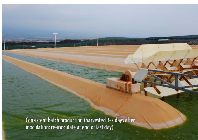
Figure 15. Cellana's large-scale hybrid cultivation system in Kona, Hawaii.
