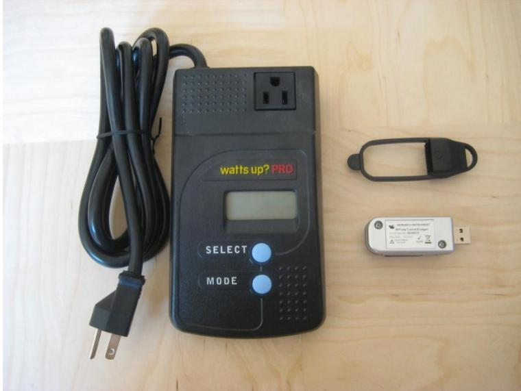
**Figure 24. Watts Up Pro Power Meter and USB Track-It Data Logger**
