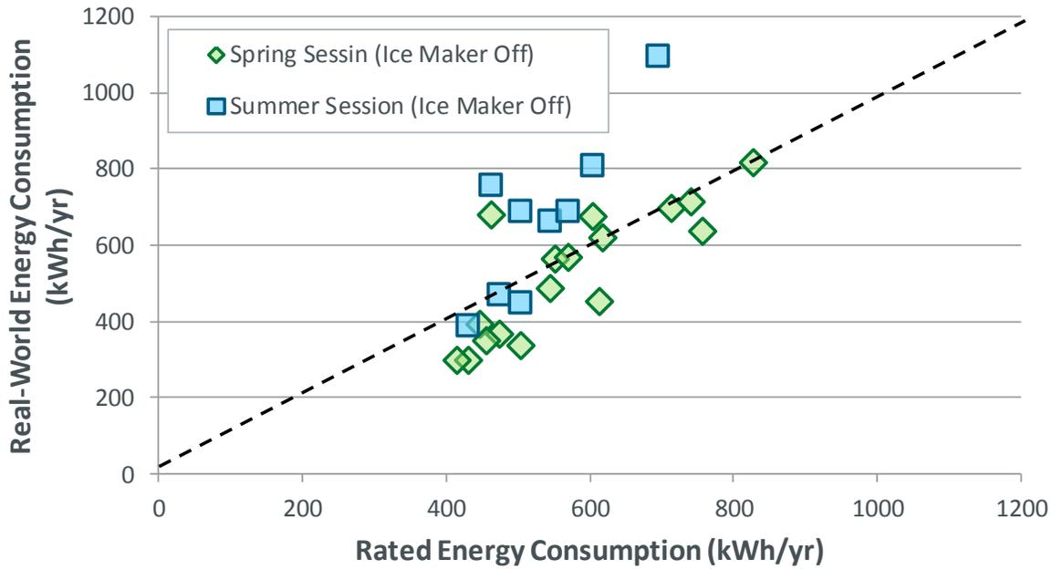
Note: Real-world energy consumption represents the measured annual energy consumption during the “ice maker off” period. Points above the dashed line indicate real-world energy consumption greater than the rated value.
