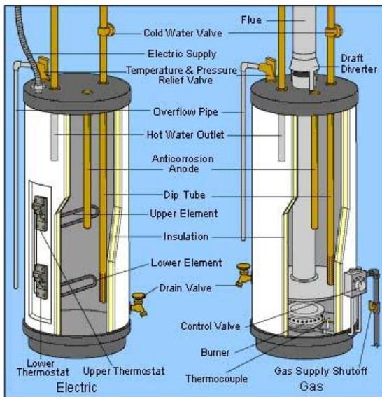
**Figure 5: Components of storage water heaters – electric and gas (Source: [www.theplumbinginfo.com](http://www.theplumbinginfo.com))**
