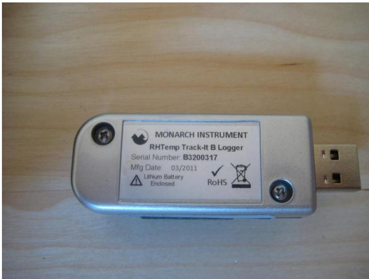
**Figure 25. USB Track-It Data Logger**
