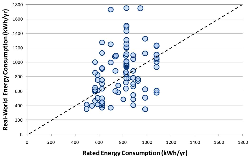
Note: Points above the dashed line indicate real-world energy consumption greater than the rated value. Data points represent raw data from the PNNL study.
