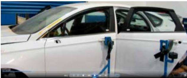
Side Door Glass - Door Slam Durability Test
