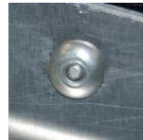
Where SPR's could not be used in the BIW and closure joints due to single side access, insufficient gun clearance, or base material issues, flow screws, Riv-Tac, and Huck rivets were used along with structural adhesive.
