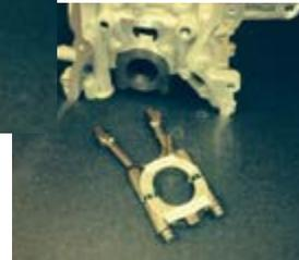
Carbon Fiber upper + Aluminum lower Cam carrier
