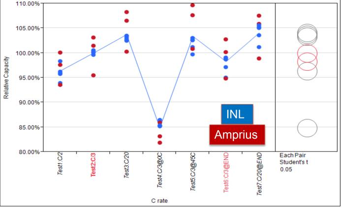
Capacity about 85% at 0°C relative to room temperature, 103% at 45°C
