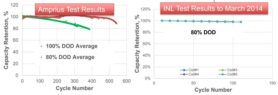
18 2.3Ah pouch cells were tested at Amprius and
