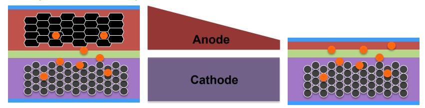
Amprius' growth-rooted silicon nanowires enable sillicon to swell and contract successfully, without compromising the battery's mechanical stability
