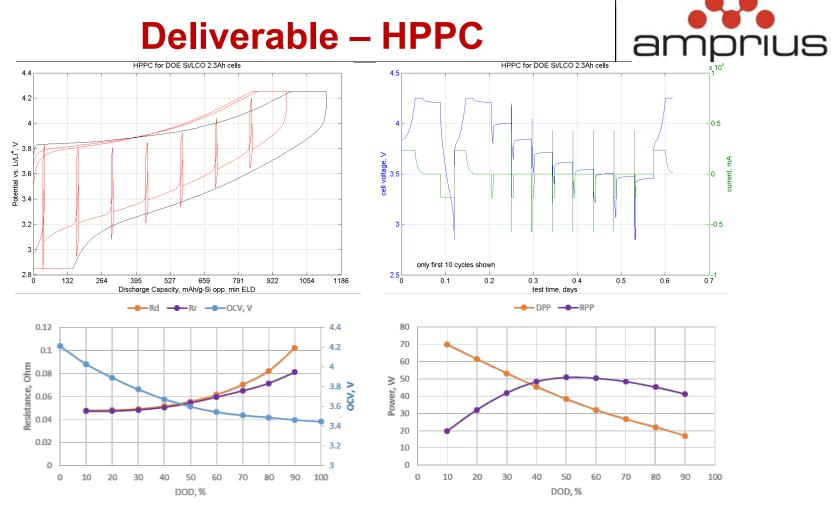
Amprius cells passed the HPPC test on all 9 discharge segments without hitting the voltage limits
