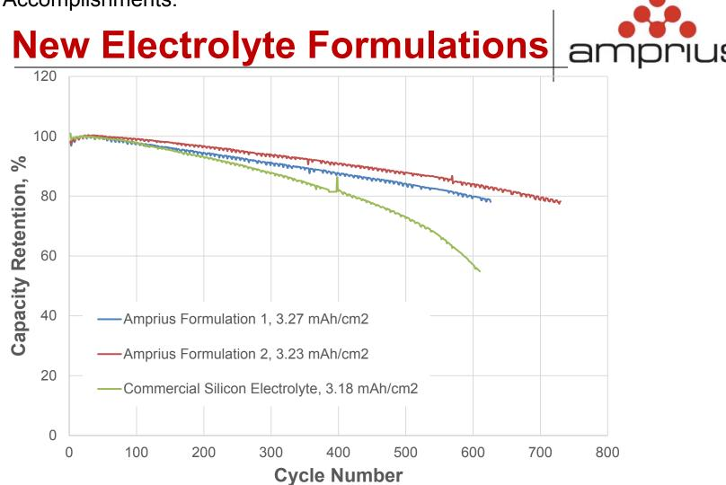
Cycle life in Si/LCO cells was increased to 700 cycles
