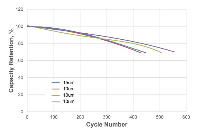
Cycle life in full cell data is not affected by foil thickness
