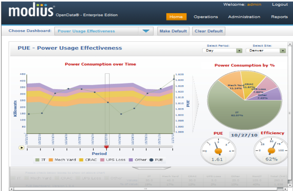
Figure 8. Dashboard for PUE, and Energy Use over Time and by End Use (Courtesy of Modius)
