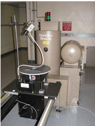
During GBI operations, a source is moved pneumatically to the top of a transfer tube, where it is captured and held in place via a suction cup and vacuum to allow instrument calibration.
