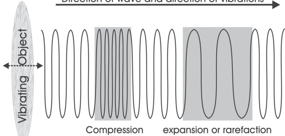
Molecules are compressed or pushed closer together.
