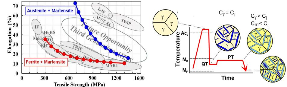
• Alloying, processing, microstructural evolution and mechanical properties inter-relationships are being studied.
