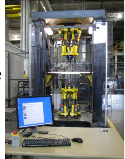
F3T system at Ford, with 400mm x 400mm work space (TRL4)
