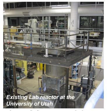
\*Different from New Bench Reactor with respect to the size and material of construction, which limits the operating temperature. Solid feed rate is limited ( $\sim 0.5 \text{ kg/hr}$ ).
