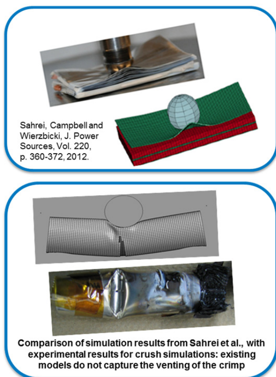
Figure IV - 103: Point of failure of a fully discharged cell coincides with the point of test, where as that for a fully charged cell is significantly different
