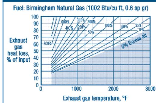
For natural gas-based systems, the amount of heat contained in the flue gases as a percentage of the heat input in a heating system can be estimated by using Figure 1. Exhaust gas loss or waste heat depends on flue gas temperature and its mass flow, or in practical terms, excess air resulting from combustion air supply and air leakage into the furnace. The excess air can be estimated by measuring oxygen percentage in the flue gases.
