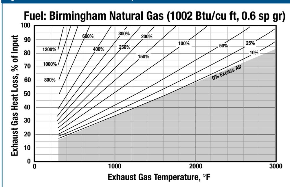
This makes it obvious that the temperature of a process, or more correctly, of its exhaust gases, is a major factor in its energy efficiency. The higher that temperature, the lower the efficiency.
