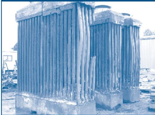
Problem areas for indirectly heated systems where heating media such as air, steam, or hot liquids are used include scale, dirt, oxide film, or fouling on the heat transfer surfaces that are in contact with the heating medium.
