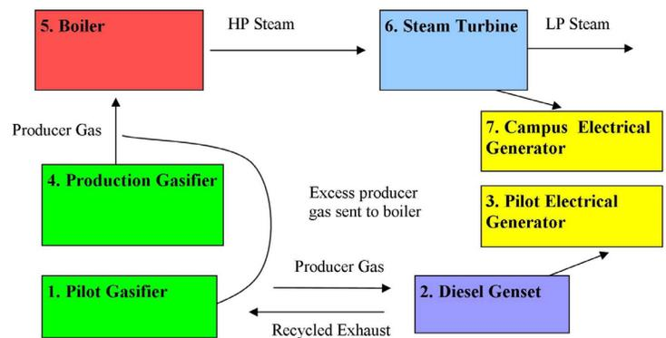
Energy-flow schematic for use of a producer gas-powered genset.
