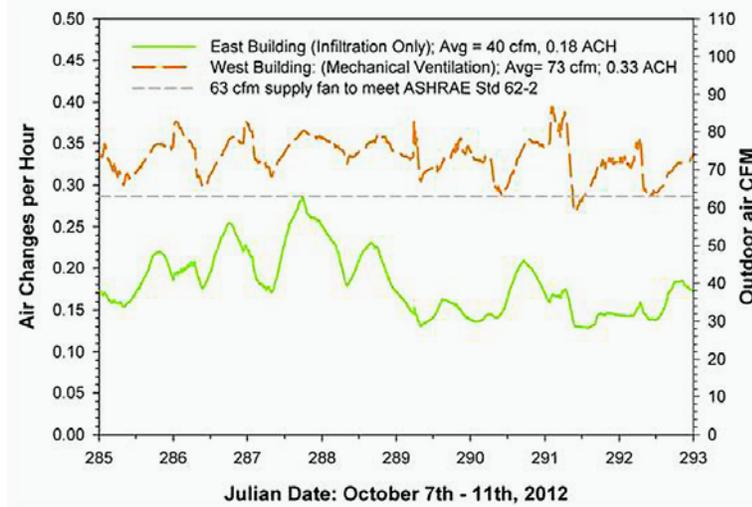
CO<sub>2</sub> is used as a tracer gas to measure infiltration in near real time.
