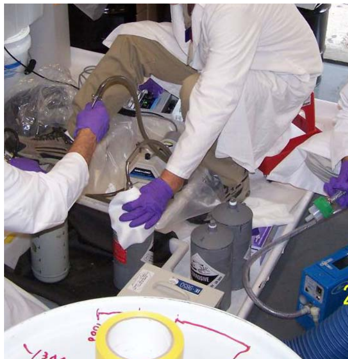
Figure C.4. Transfer operations in a large floor pan. Transfer operations should be performed on a table under a fume hood.
