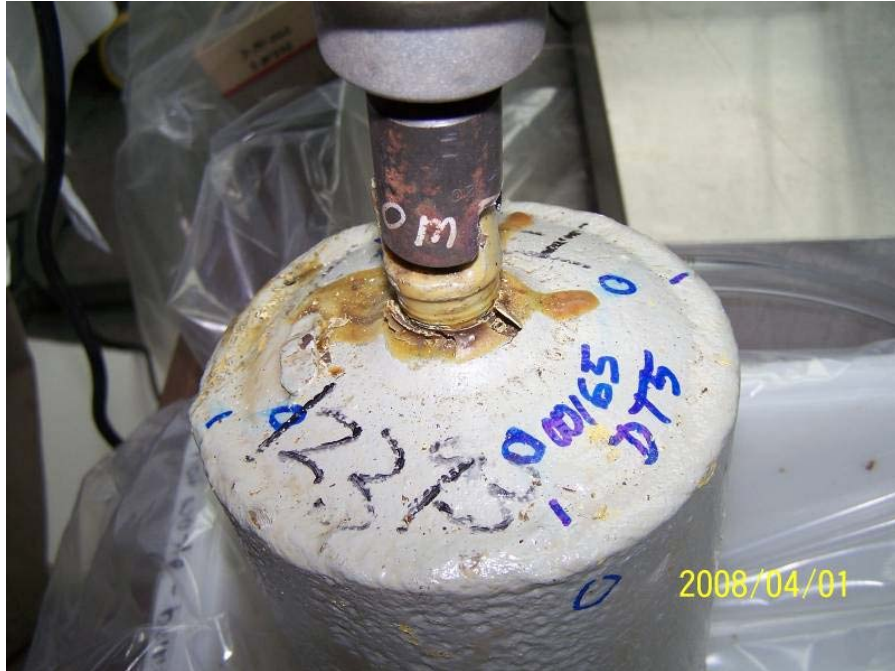
Figure C.1. Impact wrench. Note the slotted socket tool.
