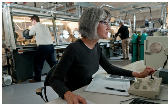
Figure V - 63: Argonne Post-test facility. The inert-atmosphere glovebox used for sample harvesting and analysis is shown in the background
