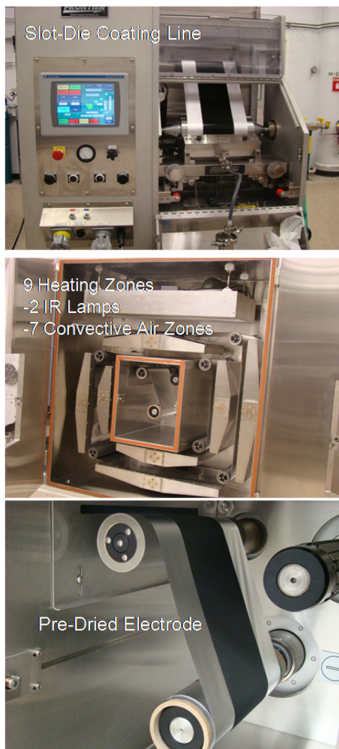
Figure V - 164: Demonstration of electrode coating via slot-die coater
