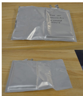
Figure V - 173: Pouch cell showing gas generation during aging process
