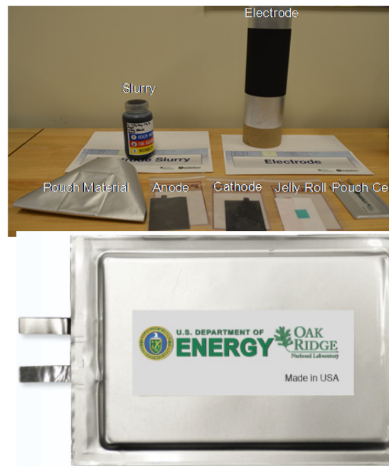
Figure V - 166: Intermediate samples in battery manufacturing and finished pouch cell
