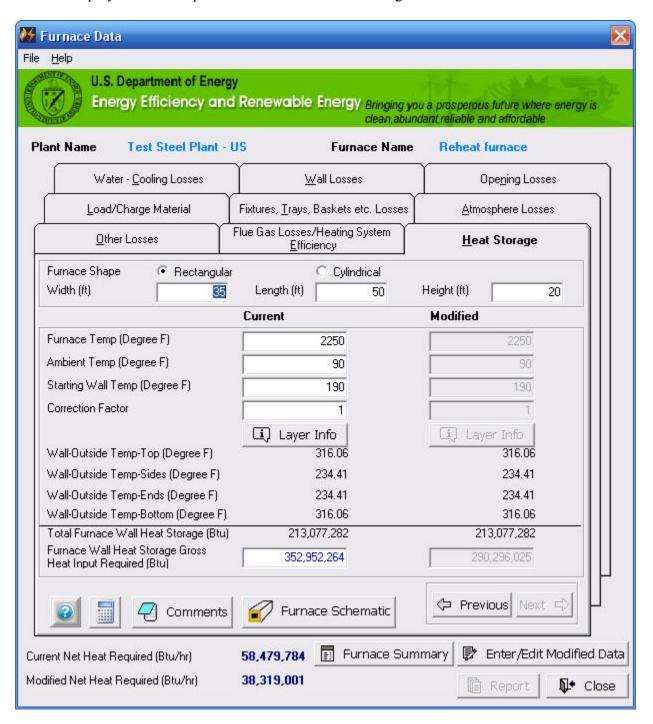
• Enter the **Information** about furnace shape, dimensions and temperatures.
