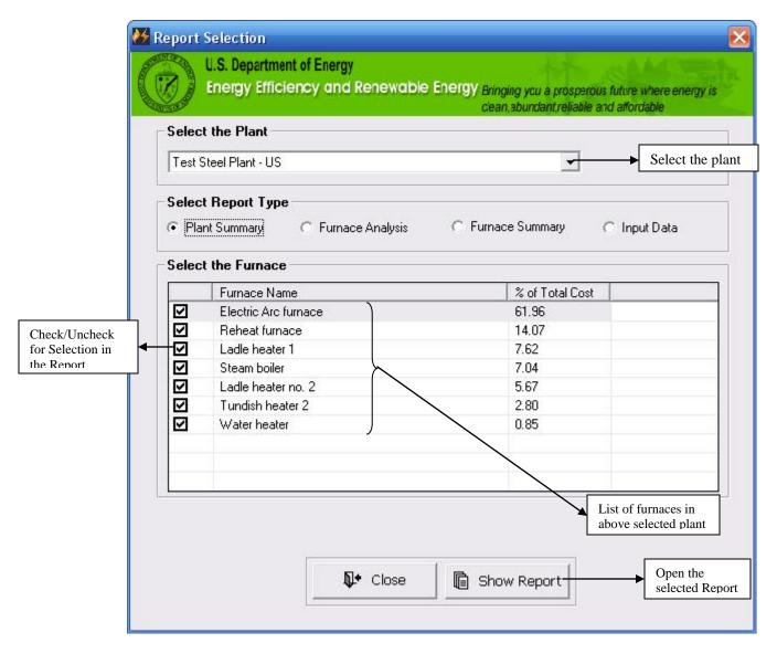
• Select a **Plant** from the drop down list. All furnaces of the selected plant will be displayed as a list with the percentage of total cost of the plant.
