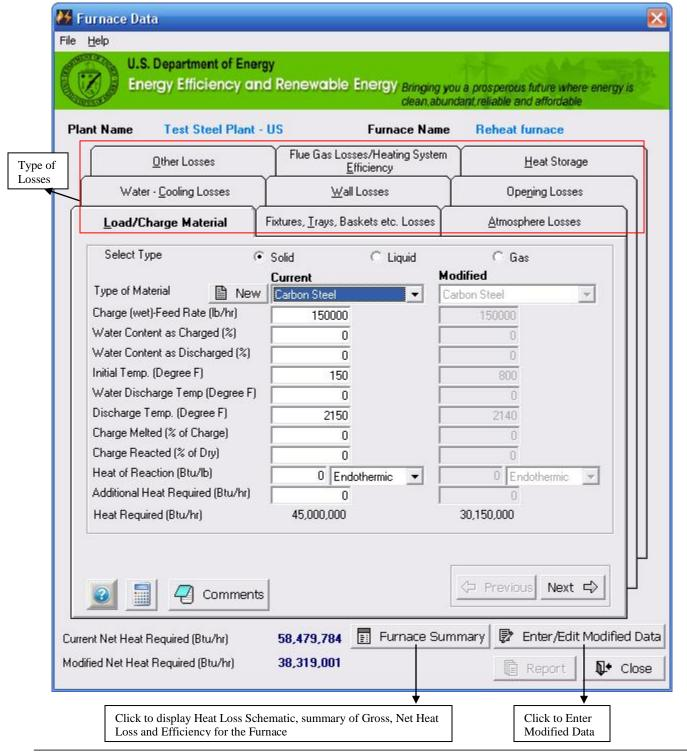
There are nine tabs that represent commonly encountered losses (mentioned below) in a furnace. The screens are designed for use with fuel fired furnaces but can also be used for electrically heated (i.e. induction, resistance, arc/plasma or other) furnaces.
