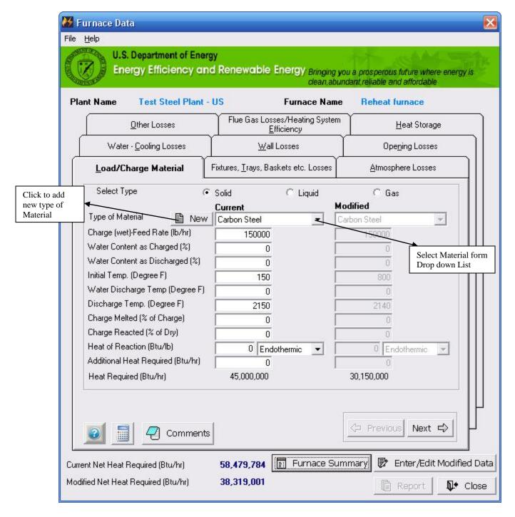
• Select the **Type** of material (i.e. Solid, Liquid, and Gas) for load charge.
